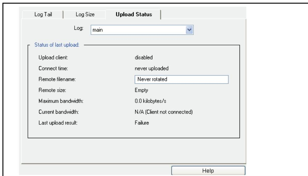
2. Under **Status of Last Upload**, check the appropriate status information displayed in the **Upload client** field.
