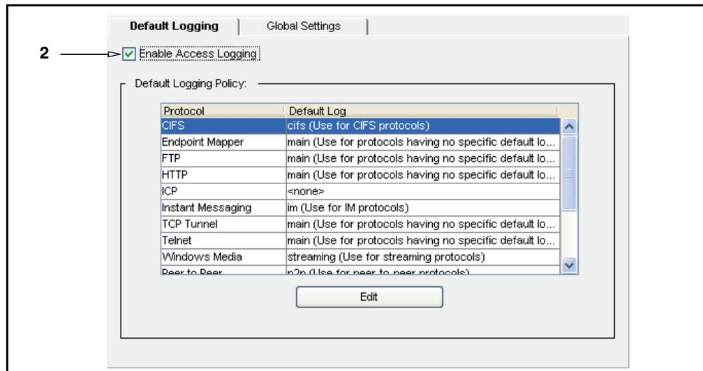
2. Select **Enable** to enable access logging or deselect it to disable access logging.
