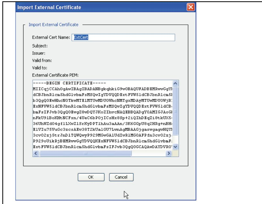
4. Enter the name of the external certificate into the **External Cert Name** field and paste the certificate into the **External Certificate** field. Be sure to include the `-----BEGIN CERTIFICATE-----` and `-----END CERTIFICATE-----` statements.
