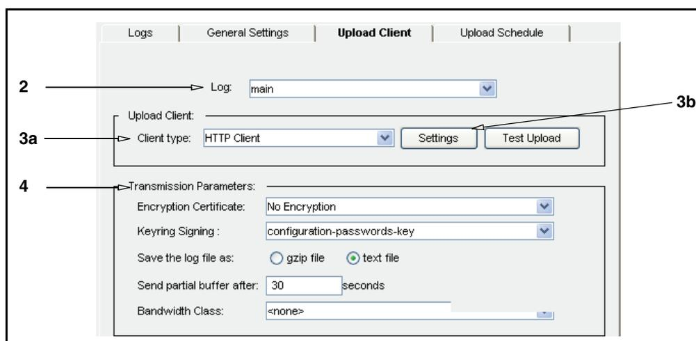
2. From the **Log** drop-down list, select the log facility to configure. The facility must exist before it displays in this list.
