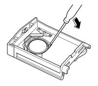
5. Put in the new battery (CR1620 or equivalent) with the positive pole (+ ) facing down.
