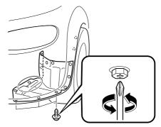
3. Turn the center section of the plastic retainers counterclockwise and remove them, then remove the mudguard.
