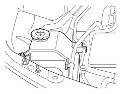
Use plain water if washer fluid is unavailable. But use only washer fluid in cold weather to prevent it from freezing.
