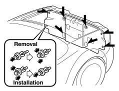
2. On the side the bulb is to be replaced, pull the center section of the plastic retainers and remove them, then remove the trunk side trim.
