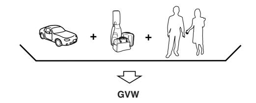
GVW (Gross Vehicle Weight) is the Vehicle Curb Weight + cargo + passengers.
