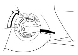
9. Turn the ignition switch from the ACC position to the START position and hold (up to 10 seconds at a time) until the engine starts.
