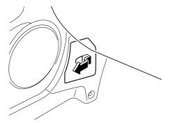
3. Pull the fuse straight out with the fuse puller provided on the inside of the engine compartment fuse block cover.
