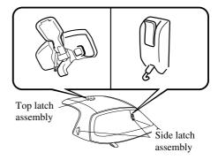
9. Align the rear deck latches with the rear deck studs and set the hardtop squarely onto the body.
