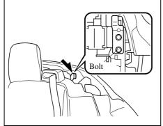
3. Use the eyebolt to get enough torque on the short leg of the Allen wrench and turn the Allen wrench 4 times counterclockwise.
