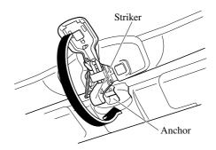
12. Pull the levers and fully release the side latches.
