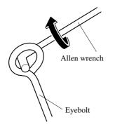
4. Disconnect the eyebolt from the Allen wrench leaving the Allen wrench in place, and insert the threaded end of the eyebolt in the hole directly above the Allen socket and tighten it clockwise two full turns.
