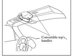
6. Sitting in a seat, grasp the convertible top's handles, and press the convertible top against the windshield. Move the top latch slowly to make sure the anchor engages with the striker, then rotate the top latch to the lock position until a click sound is heard.
