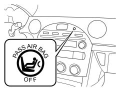
If the passenger weight sensors are working properly, the indicator light illuminates when the ignition switch is turned to the ON position. After about 6 seconds it goes out.
