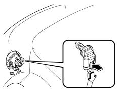
6. Install the new socket and bulb assembly in the reverse order of removal.
