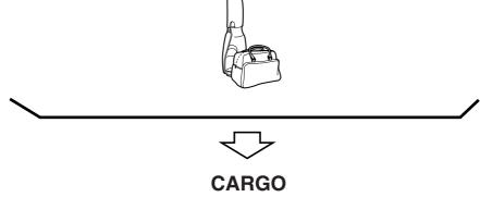
**Cargo Weight** includes all weight added to the Base Curb Weight, including cargo and optional equipment. When towing, trailer tongue load or king pin weight is also part of cargo weight.
