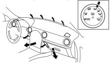
You will feel more comfortable by using the OPEN MODE when opening the roof.
