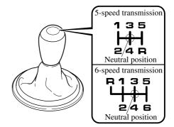
The vehicle is equipped with either a 5speed or 6-speed manual transmission. The shift pattern for each is shown above.
