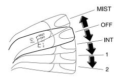
Turn the wipers on by pulling the lever down. MIST — Mist
