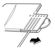
4. Insert the new battery (CR2025 or equivalent) with the positive pole (+) facing the (+) mark on the cap.
