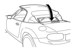
8. After the convertible top has been folded down, press the back end of the folded down convertible top until a click sound is heard, then the front end. Lightly rock the retracted convertible top to make sure it is securely locked.
