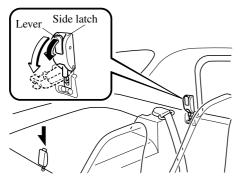
9. After the side latches are fully released, release the lever.
