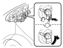
3. Install the new socket and bulb assembly in the reverse order of removal.
