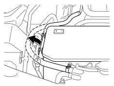
2. Remove the battery cover from its right side.
