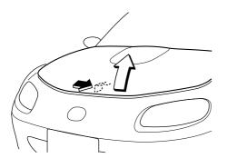
3. Grasp the support rod in the padded area and secure it in the stay hole indicated by the arrow to hold the hood open.
