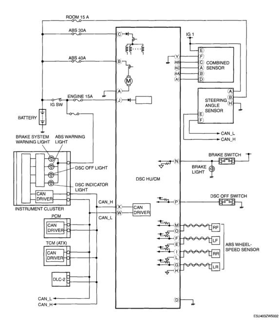
**Fig. 2: DSC System Wiring Diagram** Courtesy of MAZDA MOTORS CORP.
