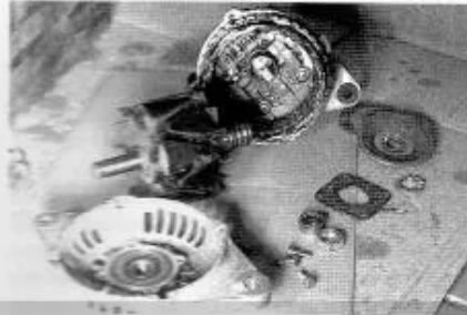
8/8 The dismantled alternator.
