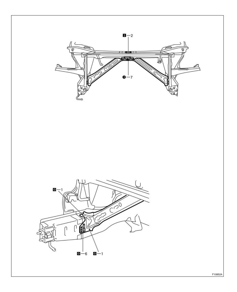
3. APPLYING SEALER TO THE ENGINE COMPARTMENT (See page PC-1)
