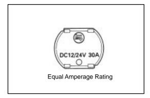
HINT: If replacing the circuit breaker, be sure to replace it with a breaker with an equal amperage rating.
