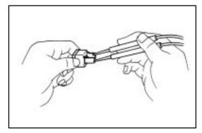
(b) Using an ohmmeter, check that there is continuity between both terminals of the circuit breaker. If continuity is not as specified, replace the circuit breaker.
