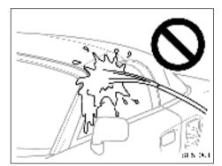
Spray water on the side windows or top seals from above, at a  $45^{\circ}$  angle to the ground.
