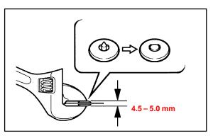
D. Check to be sure that the male pin of the Tongue Plate Stopper has become deformed evenly in the hole of the female part and is firmly held to the belt webbing. (See illustrations.)
