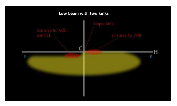
For older U.S. headlamps, the ones with the three lens bumps or the spirit level, you will have to do your best to place the left edge of the low beam "hot spot" on (or slightly overlapping) the vertical line extending down from the **C** mark in front of the lamp you're aiming, so the correctly-aimed beam (vertically and horizontally) looks like this:
