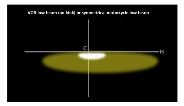
For older U.S. headlamps, the ones with the three lens bumps or the spirit level, you will have to do your best to place the top edge of the low beam's high-intensity "hot spot" on the applicable horizontal line per the table above.
