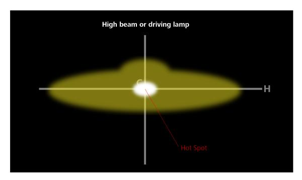
Pay attention to just one lamp at a time. It is best to unplug the headlamp you are not working on, so light from its beam pattern doesn't mislead you or make it hard to keep track of hot spots and cutoffs. Also be sure to disconnect or cover the adjacent high/low beam lamp when you are aiming its high-beam-only neighbour.
