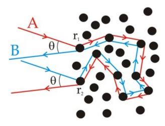
Propagation of two rays in a random medium. Since one can be obtained from the other by time inversion, they interfere coherently when the angle  $\theta$  goes to zero.
