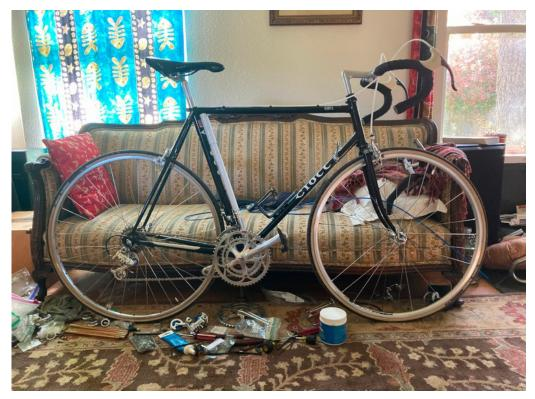
She has recently been joined by that 1984 Ciocc, which I snagged at a steep discount on Ebay and built up. It has Modolo professional brakes and a Campy triple crank. The gear cluster is period, being a 7-
