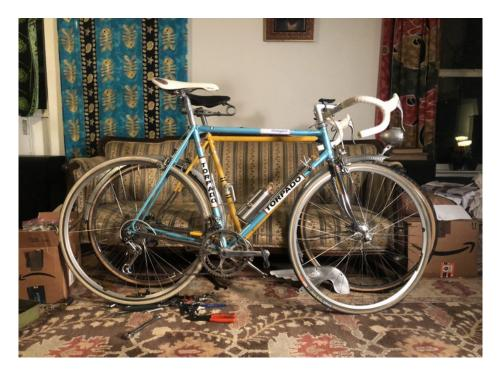
That's not a project bike, that is my old Torpado I have had since 1987. It has been very good to me over the years. The only change I made when I moved here was the rear derailleur, which needed that long cage to allow a 30T on the back. You don't see many Campy Super Records with that long cage. Everything else is original equipment, including that Flight saddle. The chrome on the frame is nearly flawless after 37 years, and you can be sure I have never left her out in the rain for a second.
