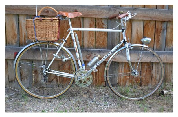
That's another Peugeot picnic bike, from about 1970. I eventually found an Ideale saddle for that, making it all period. Note the triple crank in front. It is also rare to see fenders with 27" wheels. They fit very tight, since the bike was not made for fenders. It was built as a racer, but compared to the Italian racers from that period I am showing you, it wasn't much of bike. Looks great as an upscale picnic bike though. That is the first one I restored, back in about 2016.
