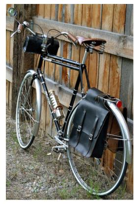
anyone like that so I just ride it myself, to the grocery store. Not something you want to leave very long in a bike rack, though, not even with a U-lock. Someone will start stripping parts off it. Note the rare Campy three-arm crank, the ribbed and corked water bottle, the hammered fenders, the Silca/Campy framefit pump, the Brooks springer saddle, the Michelin whitewalls, and the gorgeous leather saddlebags.
