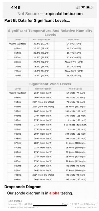
The decoded dropsonde readings. Dew point is important because when temperature and dew point are the same, moisture in the air condenses as rain. When they are within five degrees Fahrenheit of each other, the condensation usually begins.
