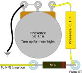
The Presence Control Circuit removes high frequencies from the NFB Circuit which boosts highs at the speaker.
