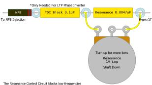
In the NFB Circuit which boosts lows at the speaker. For best results put the Resonance Control on the output transformer side of the NFB Resistor.
