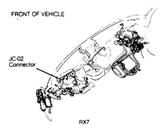
Fig. 6: Locating JC-02 Connector Courtesy of MAZDA MOTORS CORP.
