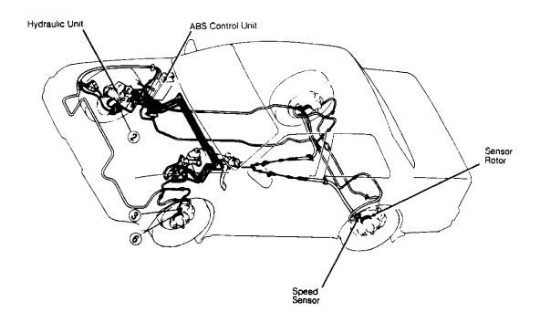
**Fig. 3: Locating ABS Components (929)** Courtesy of MAZDA MOTORS CORP.
