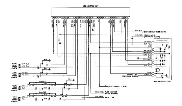
Fig. 29: Anti-Lock Brake System Wiring Diagram (929)
