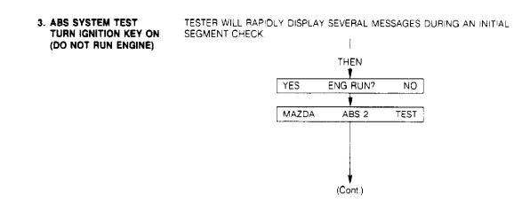
**Fig. 15: Test 3 ABS System Test** Courtesy of MAZDA MOTORS CORP.
