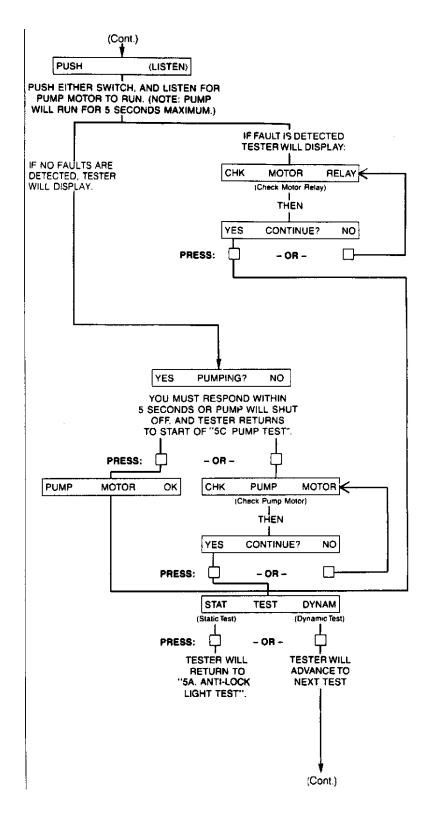
Fig. 19: Test 5C. Pump Test
