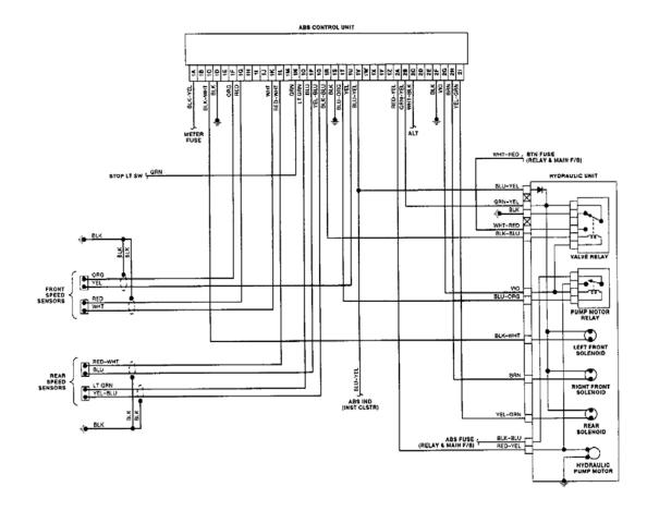
Fig. 27: Anti-Lock Brake System Wiring Diagram (Miata)
