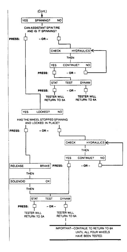
Fig. 26: 6C. Solenoid Test (4 of 4)
