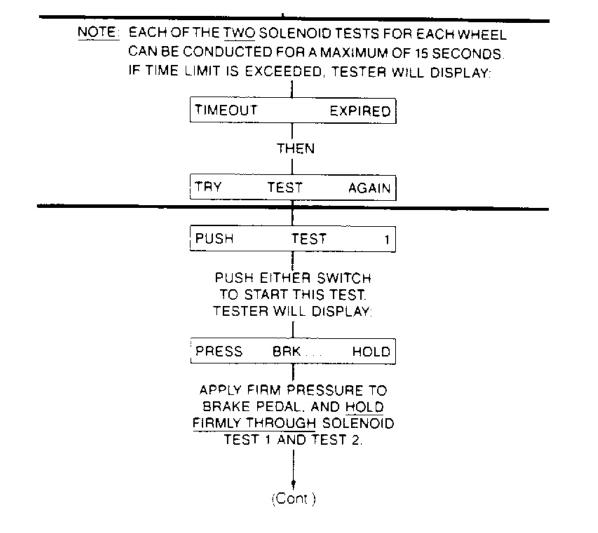
**Fig. 23: 6C. Solenoid Test (1 of 4)** Courtesy of MAZDA MOTORS CORP.
