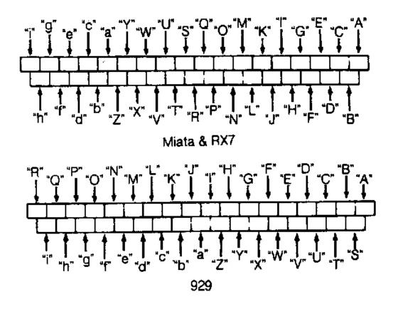
**Fig. 5: Identifying Control Unit Harness Connector Terminals** Courtesy of MAZDA MOTORS CORP.
