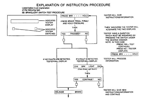
Fig. 13: Operating ABS Tester Courtesy of MAZDA MOTORS CORP.
