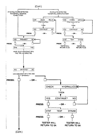
**Fig. 24: 6C. Solenoid Test (2 of 4)** Courtesy of MAZDA MOTORS CORP.
