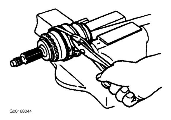
Fig. 16: Installing Boot Band Courtesy of MAZDA MOTORS CORP.
