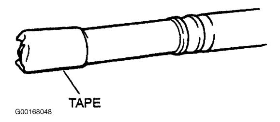
Fig. 13: Installing CV Joint Boot Courtesy of MAZDA MOTORS CORP.
