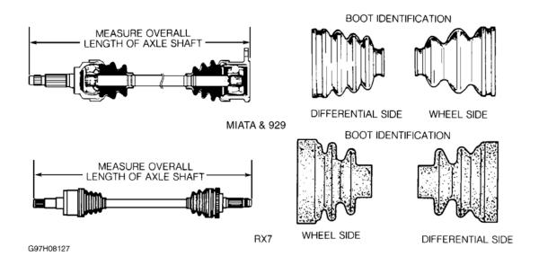
Fig. 12: Measuring Axle Shaft & Identifying Boots Courtesy of MAZDA MOTORS CORP.
