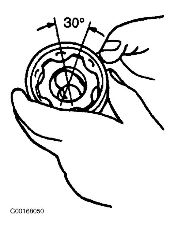
Fig. 10: Separating Inner Ring From Cage Courtesy of MAZDA MOTORS CORP.
