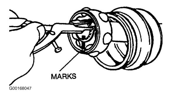
Fig. 7: Removing Snap Ring Courtesy of MAZDA MOTORS CORP.
