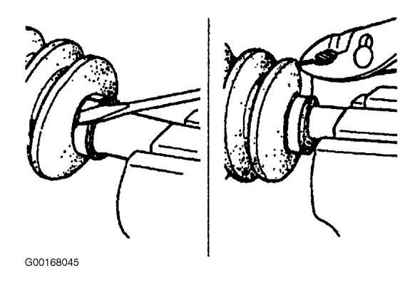
Fig. 5: Removing Boot Band Courtesy of MAZDA MOTORS CORP.
