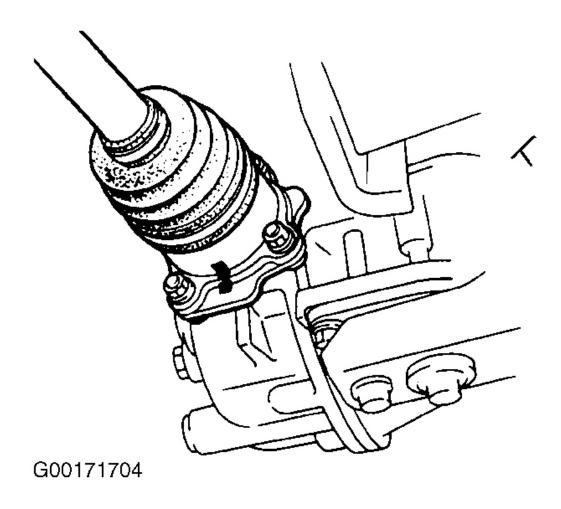
Fig. 2: Identifying Differential-To-Axle Shaft Flange Mark Courtesy of MAZDA MOTORS CORP.
