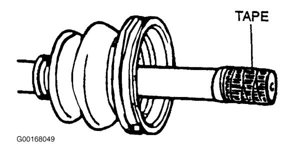
Fig. 11: Removing CV Joint Boot Courtesy of MAZDA MOTORS CORP.
