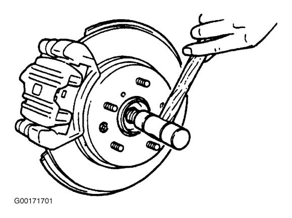
Fig. 3: Removing Axle Shaft From Hub Assembly Courtesy of MAZDA MOTORS CORP.
