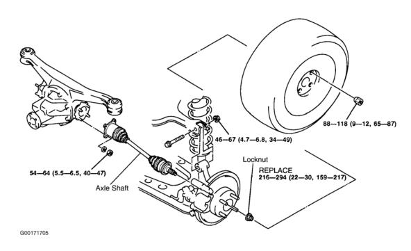
Fig. 1: Removing Axle Shaft Courtesy of MAZDA MOTORS CORP.
