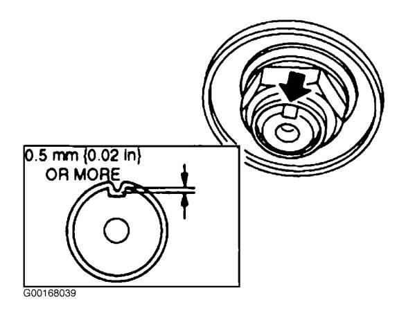
Fig. 4: Installing Axle Shaft Lock Nut Courtesy of MAZDA MOTORS CORP.
