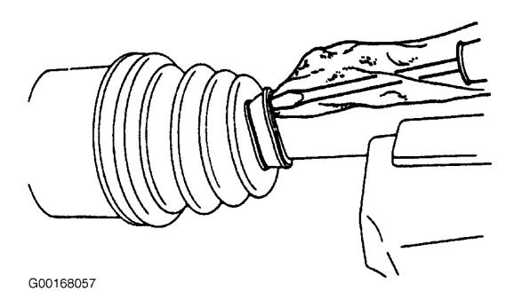
Fig. 15: Releasing Trapped Air Courtesy of MAZDA MOTORS CORP.
