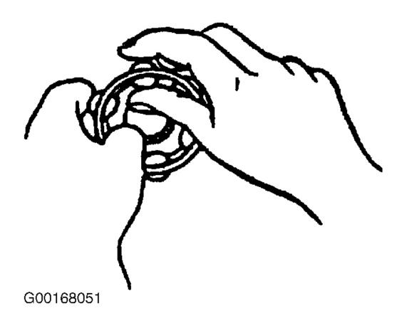
Fig. 9: Removing Balls From Inner Ring Courtesy of MAZDA MOTORS CORP.
