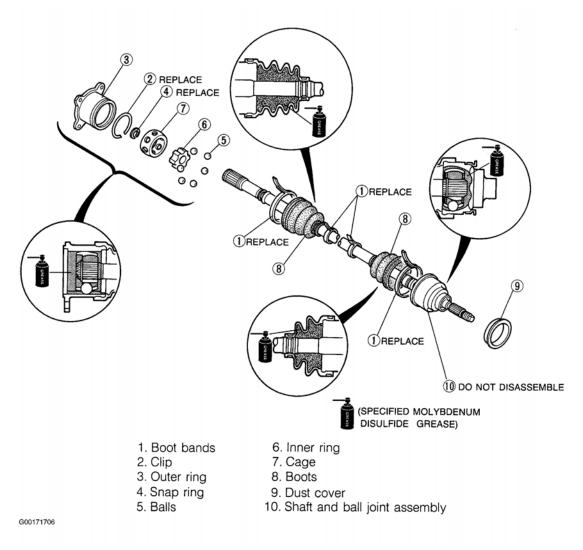
Fig. 8: Exploded View Of Axle Shaft Assembly Courtesy of MAZDA MOTORS CORP.
