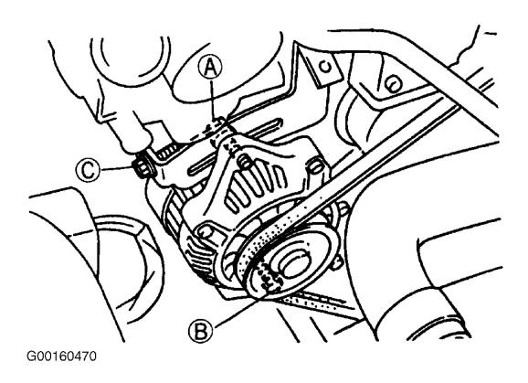
Fig. 2: Adjusting Alternator Belt Courtesy of MAZDA MOTORS CORP.
