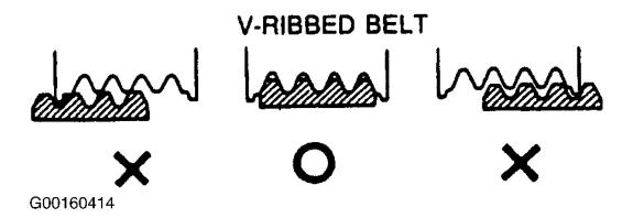
Fig. 1: Identifying Correct Belt Mounting Courtesy of MAZDA MOTORS CORP.
