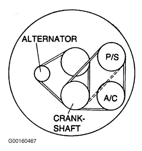
Fig. 5: Identifying Drive Belt Routing & Deflection Check Point (1 Of 3) Courtesy of MAZDA MOTORS CORP.
