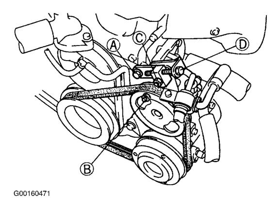
Fig. 3: Adjusting A/C Compressor & Power Steering Pump Belt Courtesy of MAZDA MOTORS CORP.
