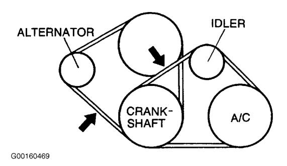
Fig. 7: Identifying Drive Belt Routing & Deflection Check Point (3 Of 3) **Courtesy of MAZDA MOTORS CORP.**
