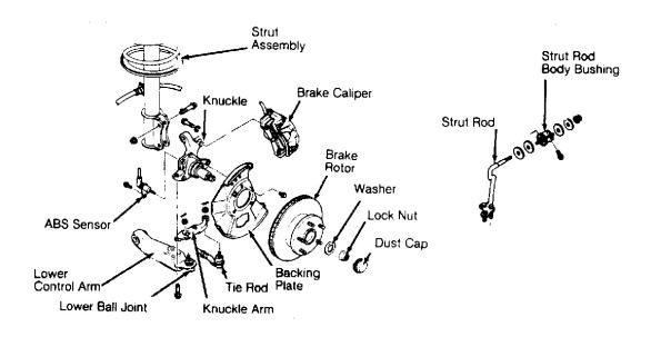
Fig. 4: Exploded View of Front Suspension (MPV & 929) Courtesy of MAZDA MOTORS CORP.
