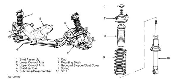
Fig. 1: Exploded View of Front Suspension (Miata) Courtesy of MAZDA MOTORS CORP.
