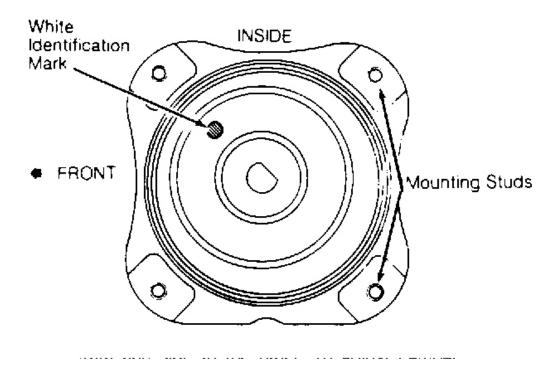
Fig. 6: Positioning Strut for Installation (MPV, RX7 & 929) Courtesy of MAZDA MOTORS CORP.
