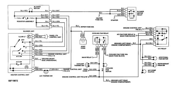
Fig. 7: Manual Heater-A/C System Wiring Diagram (1992)
