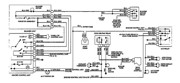
Fig. 5: Manual Heater-A/C System Wiring Diagram (1990)
