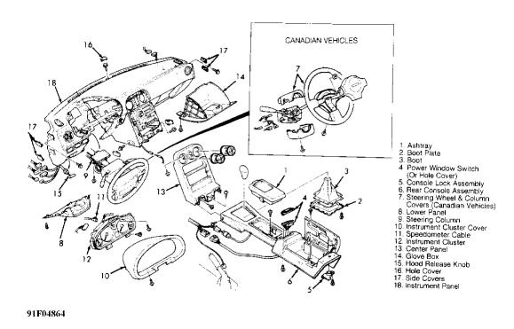
Fig. 4: Exploded View of Instrument Panel Courtesy of MAZDA MOTORS CORP.
