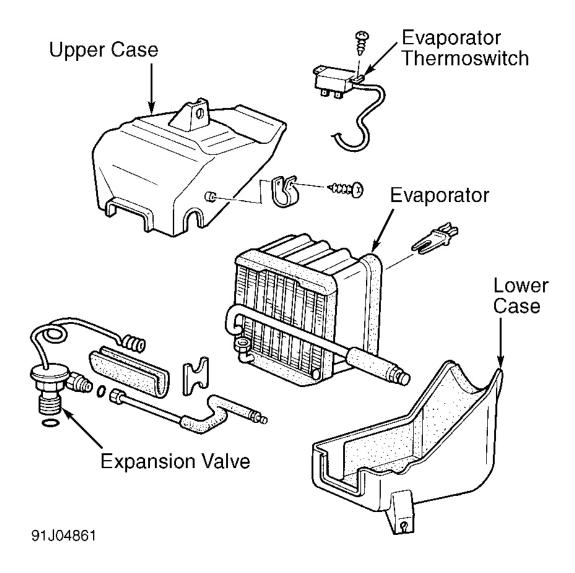
Fig. 3: Exploded View of Evaporator Case Courtesy of MAZDA MOTORS CORP.
