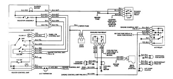
Fig. 6: Manual Heater-A/C System Wiring Diagram (1991)
