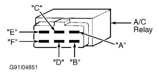
Fig. 2: A/C Relay Connector Terminal ID Courtesy of MAZDA MOTORS CORP.
