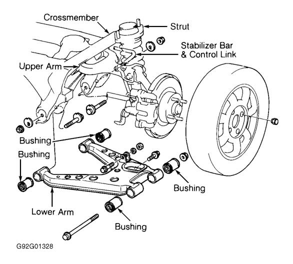
Fig. 1: Exploded View of Rear Lower Arm Assembly Courtesy of MAZDA MOTORS CORP.
