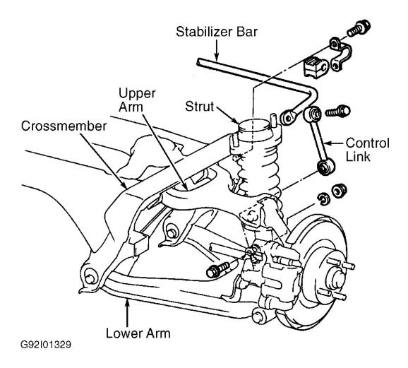
Fig. 2: Exploded View of Rear Stabilizer Bar & Control Link Courtesy of MAZDA MOTORS CORP.
