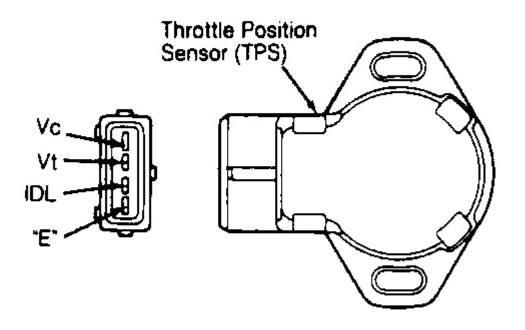
Fig. 3: TP Sensor Connector Terminal ID (A/T) Courtesy of MAZDA MOTORS CORP.
