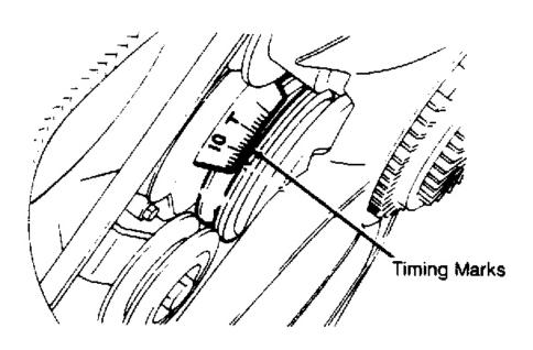
Fig. 1. Locating Ignition Timing Marks
