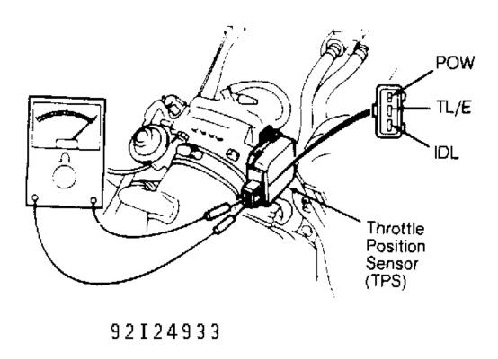
Fig. 4: TP Sensor Connector Terminal ID (M/T) Courtesy of MAZDA MOTORS CORP.
