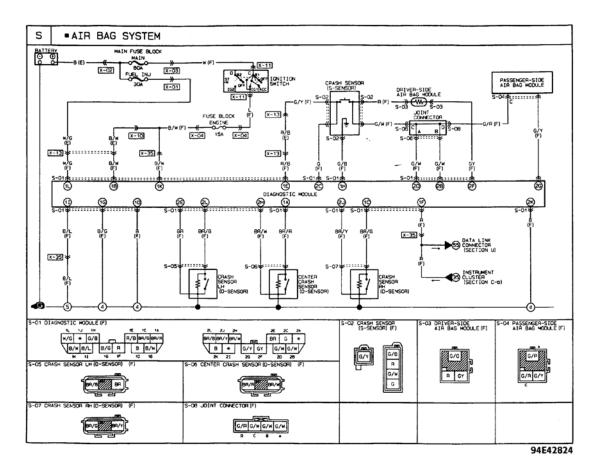
Fig. 14: Air Bag System Wiring Diagram Courtesy of MAZDA MOTORS CORP.
