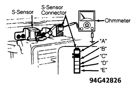
Fig. 9: Identifying S-Sensor Connector Terminals Courtesy of MAZDA MOTORS CORP.
