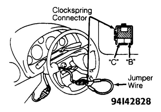
Fig. 11: Identifying Clockspring Connector Terminals Courtesy of MAZDA MOTORS CORP.
