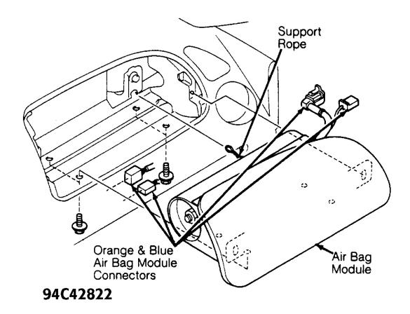
Fig. 6: Removing Passenger Air Bag Module Courtesy of MAZDA MOTORS CORP.
