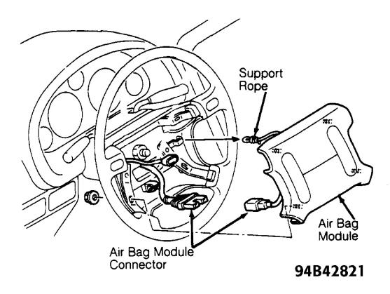
Fig. 5: Removing Driver Air Bag Module Courtesy of MAZDA MOTORS CORP.
