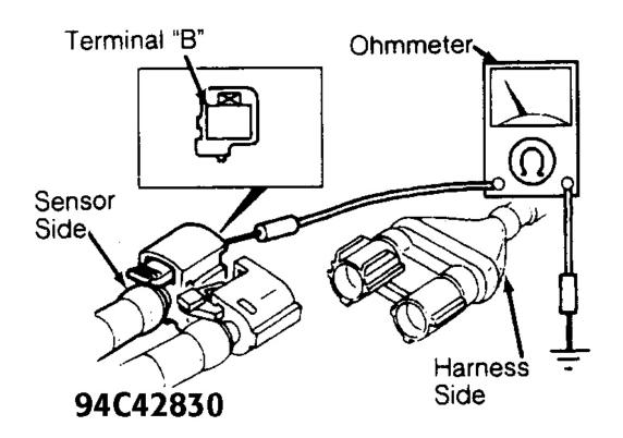
Fig. 13: Identifying D-Sensor Terminal "B" Courtesy of MAZDA MOTORS CORP.
