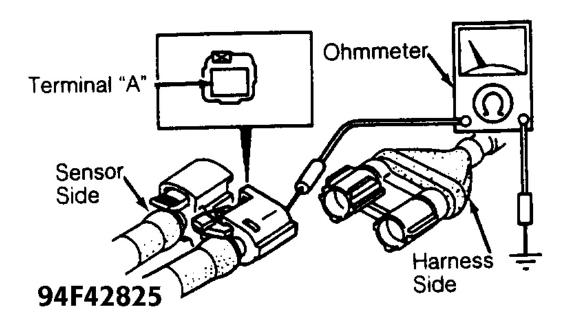
Fig. 8: Identifying D-Sensor Terminal "A" Courtesy of MAZDA MOTORS CORP.
