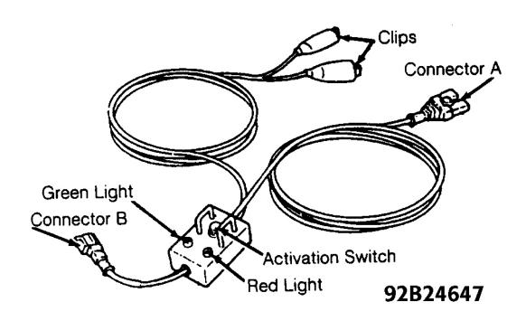
Fig. 4: Identifying Air Bag Deployment Tool Connectors Courtesy of MAZDA MOTORS CORP.
