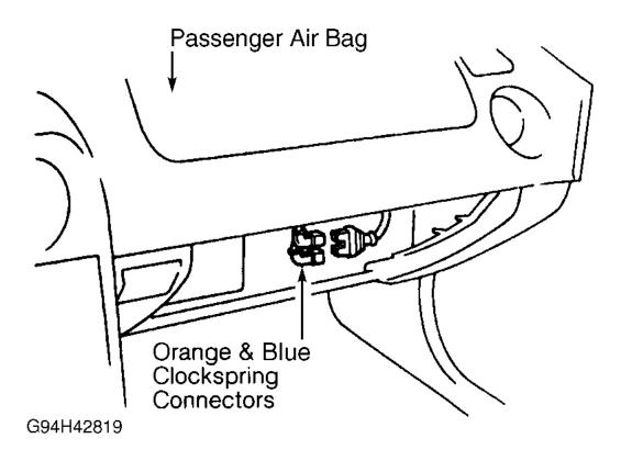
Fig. 3: Locating Passenger Air Bag Clockspring Connectors Courtesy of MAZDA MOTORS CORP.
