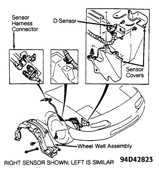
Fig. 7: Removing Front (D-Sensor)
