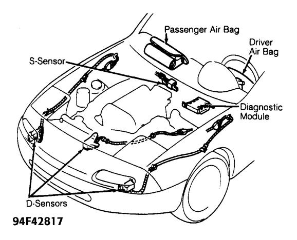
Fig. 1: Identifying Air Bag System Components Courtesy of MAZDA MOTORS CORP.
