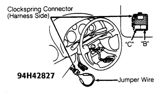
Fig. 10: Clockspring Connector Terminal ID (Harness Side) Courtesy of MAZDA MOTORS CORP.
