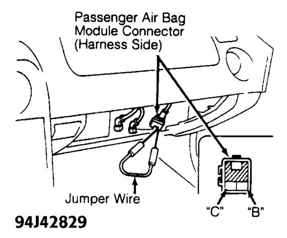
Fig. 12: Passenger Air Bag Module Connector Terminal ID (Harness Side) Courtesy of MAZDA MOTORS CORP.
