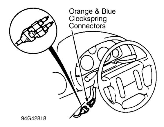
Fig. 2: Locating Driver Air Bag Clockspring Connectors Courtesy of MAZDA MOTORS CORP.
