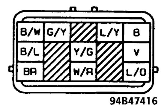
Fig. 12: Hydraulic Unit Harness Connector Terminals ID
