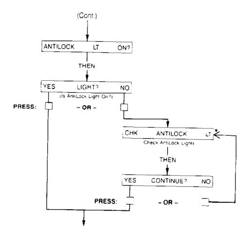
Fig. 5: Static Tests/Brake Light Switch Test (3 of 9) Courtesy of MAZDA MOTORS CORP.
