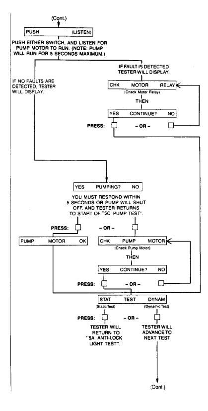
**Fig. 6: Pump Test (4 of 9)**
