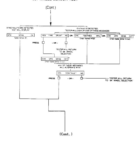
Fig. 8: Wheel Sensor Test (Cont.)/Solenoid Test (6 of 9) Courtesy of MAZDA MOTORS CORP.
