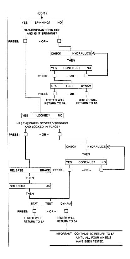
Fig. 11: Solenoid Test (Cont.) (9 of 9)
