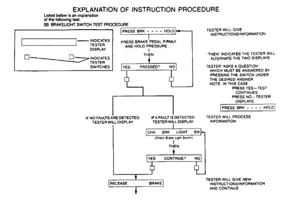
Fig. 2: Operating ABS Tester
