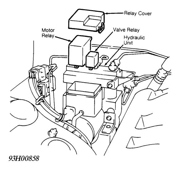
Fig. 16: Locating Valve Relay & Motor Relay
