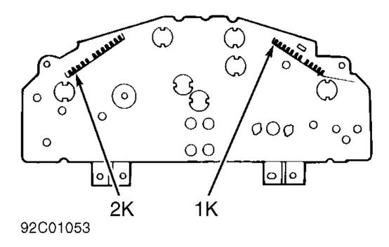
Fig. 14: Instrument Cluster Connector Terminals Courtesy of MAZDA MOTORS CORP.
