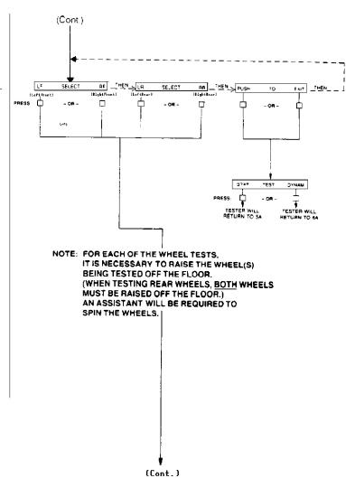
Fig. 7: Dynamic Tests/Wheel Sensor Test (5 of 9) Courtesy of MAZDA MOTORS CORP.
