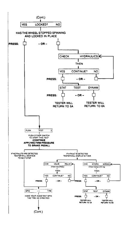
Fig. 10: Solenoid Test (Cont.) (8 of 9) Courtesy of MAZDA MOTORS CORP.
