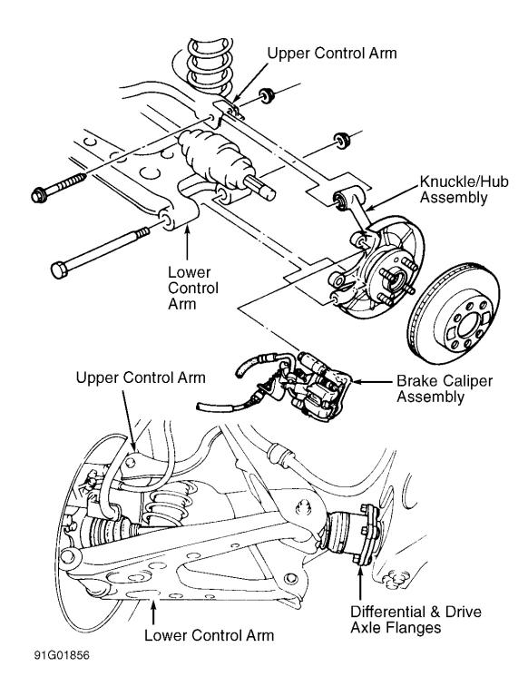
Fig. 1: Removing Rear Drive Axle & Knuckle/Hub Assembly Courtesy of MAZDA MOTORS CORP.
