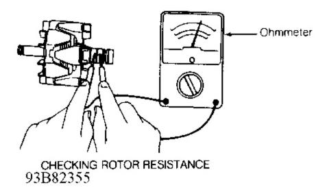
Fig. 9: Testing Generator Stator, Rotor & Brushes (5 Of 5) Courtesy of MAZDA MOTORS CORP.
