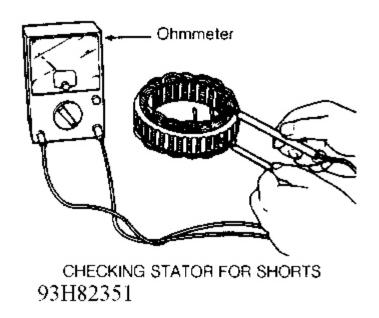
Fig. 5: Testing Generator Stator, Rotor & Brushes (1 Of 5) Courtesy of MAZDA MOTORS CORP.
