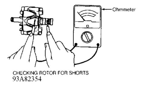
Fig. 8: Testing Generator Stator, Rotor & Brushes (4 Of 5) Courtesy of MAZDA MOTORS CORP.
