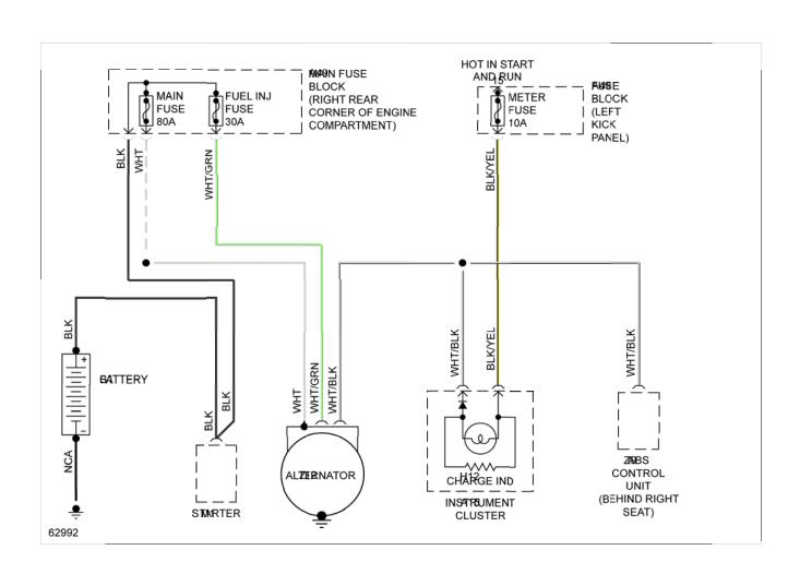
Fig. 18: Charging System Wiring Diagram (Miata)
