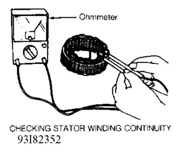
Fig. 6: Testing Generator Stator, Rotor & Brushes (2 Of 5) Courtesy of MAZDA MOTORS CORP.
