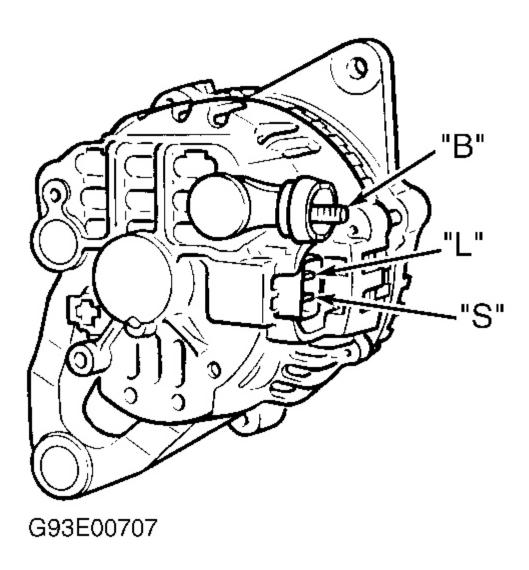
Fig. 1: Identifying Generator Terminals (Miata) Courtesy of MAZDA MOTORS CORP.
