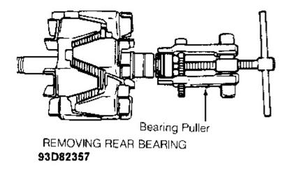
Fig. 11: Overhauling Generator (2 Of 6) Courtesy of MAZDA MOTORS CORP.
