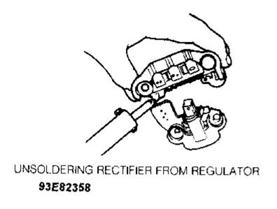
Fig. 12: Overhauling Generator (3 Of 6)
