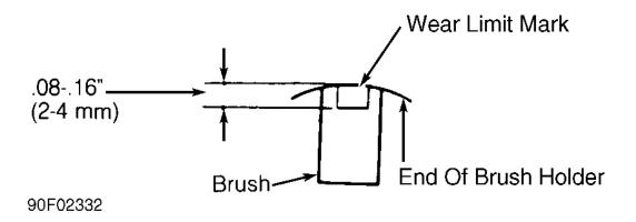
Fig. 16: Measuring Installed Depth Of Brush Courtesy of MAZDA MOTORS CORP.
