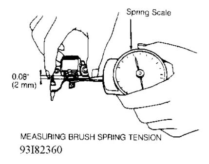
Fig. 14: Overhauling Generator (5 Of 6) Courtesy of MAZDA MOTORS CORP.
