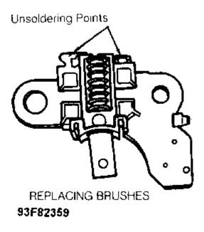
Fig. 13: Overhauling Generator (4 Of 6) Courtesy of MAZDA MOTORS CORP.
