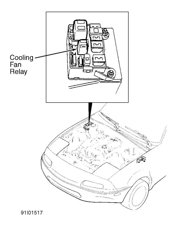
Fig. 2: Locating Cooling Fan Relay Courtesy of MAZDA MOTORS CORP.
