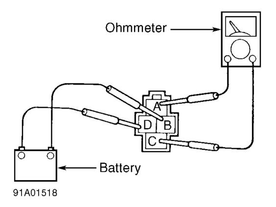
Fig. 3: Testing Cooling Fan Relay Courtesy of MAZDA MOTORS CORP.
