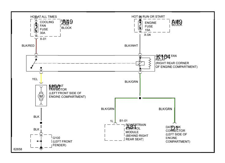
ENGINE COOLING FAN 1994 ENGINE COOLING Mazda - Engine Cooling Fans
