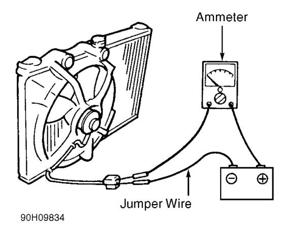
Fig. 1: Testing Cooling Fan Motor Courtesy of MAZDA MOTORS CORP.
