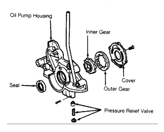
Fig. 12: Exploded View Of Oil Pump Courtesy of MAZDA MOTORS CORP.
