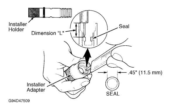
Fig. 7: Installing Valve Guide Seals Courtesy of MAZDA MOTORS CORP.
