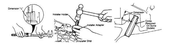
Fig. 8: Adjusting Valve Guide Installer & Installing Guide Courtesy of MAZDA MOTORS CORP.
