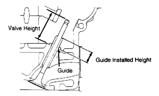
Fig. 9: Measuring Installed Valve & Guide Height Courtesy of MAZDA MOTORS CORP.
