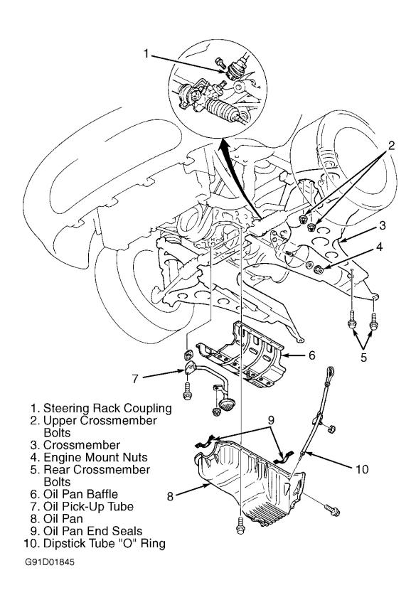
Fig. 6: Removing Crossmember & Oil Pan
