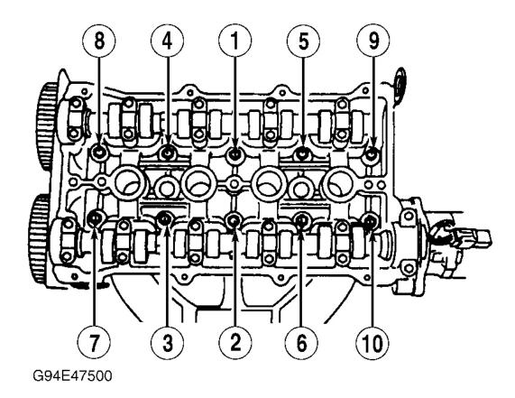
Fig. 4: Cylinder Head Bolt Tightening Sequence Courtesy of MAZDA MOTORS CORP.
