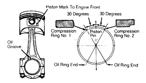
Fig. 10: Assembling Piston, Rod & Rings Courtesy of MAZDA MOTORS CORP.
