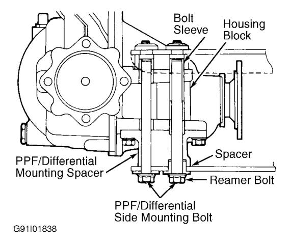
Fig. 3: Locating PPF-To-Differential Reamer Bolt, Sleeve & Spacer Courtesy of MAZDA MOTORS CORP.
