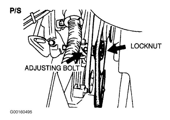
Fig. 8: Adjusting Power Steering Pump Belt (MPV) Courtesy of MAZDA MOTORS CORP.
