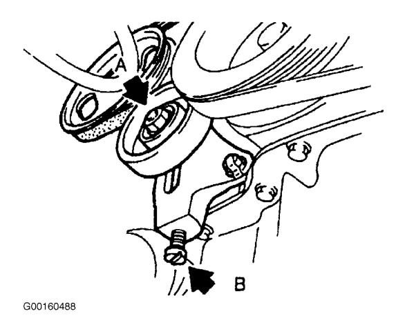
Fig. 5: Adjusting Power Steering Pump Belt (Millenia, 2.5L) Courtesy of MAZDA MOTORS CORP.
