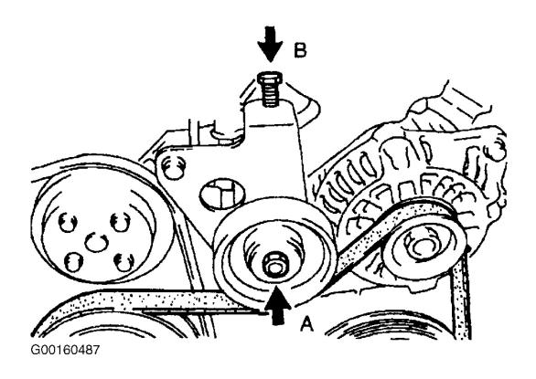
Fig. 4: Adjusting Alternator Belt (Millenia, 2.5L) Courtesy of MAZDA MOTORS CORP.
