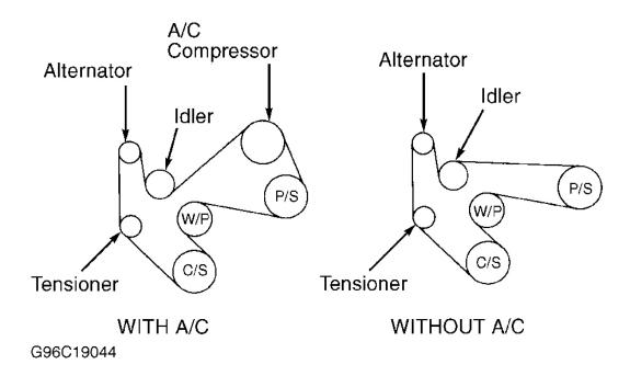
Fig. 17: Identifying Drive Belt Routing (B4000) Courtesy of FORD MOTOR CO.
