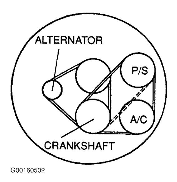
Fig. 24: Identifying Drive Belt Routing & Deflection Check Point (MX-5 Miata, 1 Of 3) Courtesy of MAZDA MOTORS CORP.
