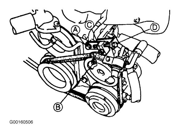
Fig. 11: Adjusting Power Steering Pump Belt (MX-5 Miata) Courtesy of MAZDA MOTORS CORP.
