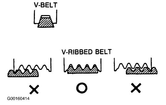
Fig. 29: Identifying Correct Belt Mounting Courtesy of MAZDA MOTORS CORP.
