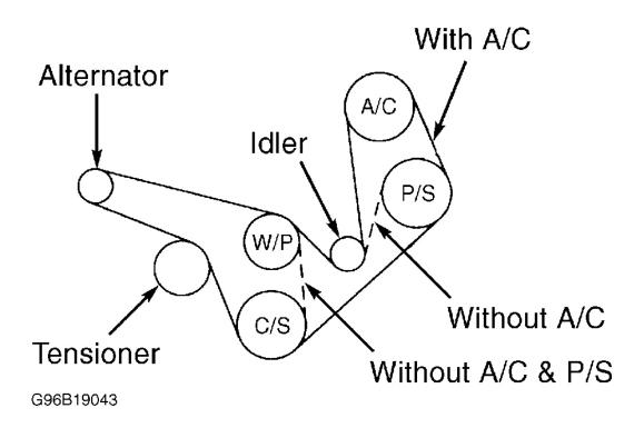
Fig. 15: Identifying Drive Belt Routing (B2300 & B2500) Courtesy of FORD MOTOR CO.
