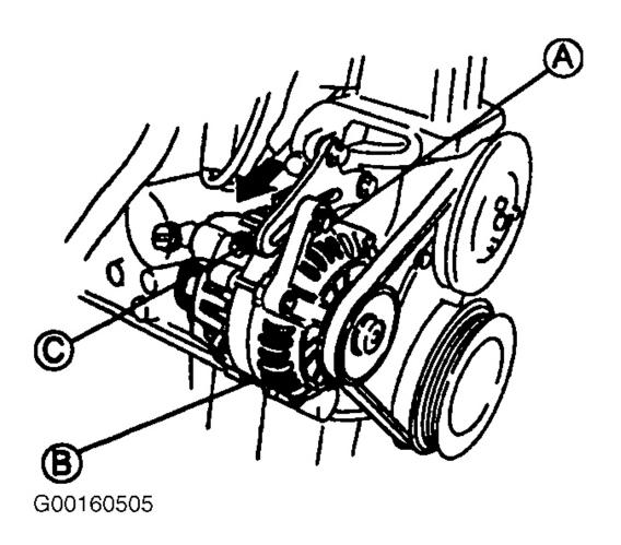
Fig. 9: Adjusting Alternator Belt (MX-5 Miata) Courtesy of MAZDA MOTORS CORP.
