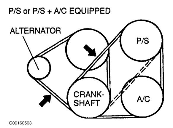
Fig. 25: Identifying Drive Belt Routing & Deflection Check Point (MX-5 Miata, 2 Of 3) Courtesy of MAZDA MOTORS CORP.
