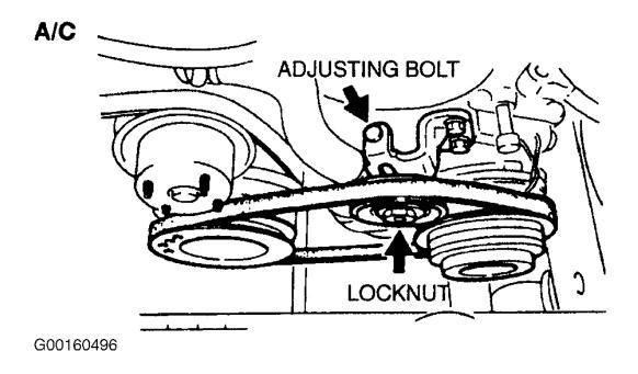
Fig. 7: Adjusting A/C Compressor Belt (MPV) Courtesy of MAZDA MOTORS CORP.
