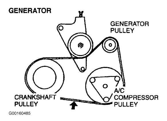
Fig. 19: Identifying Drive Belt Routing & Deflection Check Point (Millenia, 2.5L, 1 Of 2) Courtesy of MAZDA MOTORS CORP.
