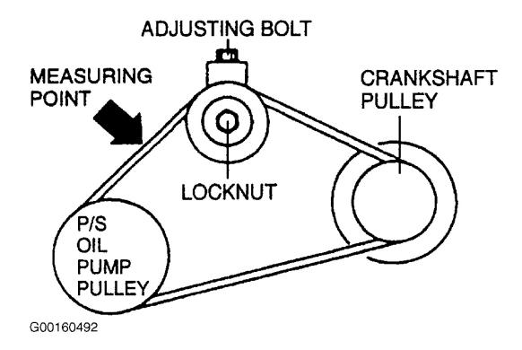
Fig. 22: Identifying Drive Belt Routing & Deflection Check Point (MPV, 2 Of 3) Courtesy of MAZDA MOTORS CORP.
