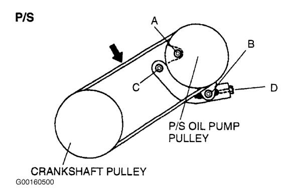
Fig. 13: Adjusting Power Steering Pump Belt (Without A/C, Protege) Courtesy of MAZDA MOTORS CORP.
