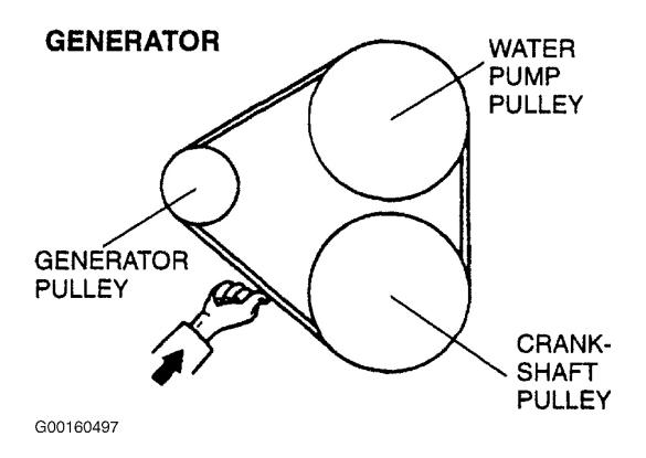
Fig. 27: Identifying Drive Belt Routing & Deflection Check Point (Protege, 1 Of 2) Courtesy of MAZDA MOTORS CORP.
