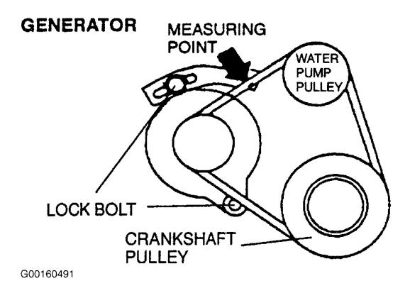
Fig. 21: Identifying Drive Belt Routing & Deflection Check Point (MPV, 1 Of 3) Courtesy of MAZDA MOTORS CORP.
