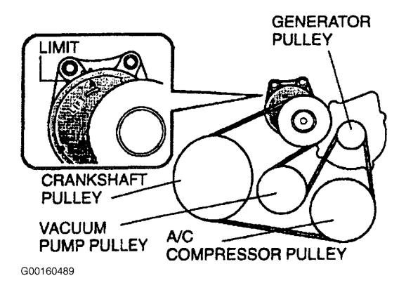
Fig. 2: Checking Alternator Serpentine Belt Tension (Millenia, 2.3L) Courtesy of MAZDA MOTORS CORP.
