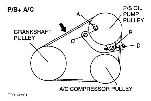
Fig. 14: Adjusting Power Steering Pump Belt (With A/C, Protege) Courtesy of MAZDA MOTORS CORP.
