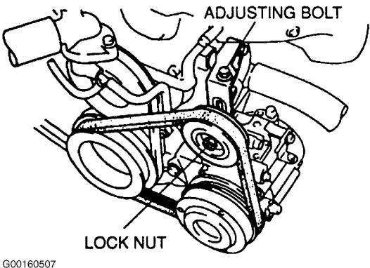
Fig. 10: Adjusting A/C Compressor Belt (MX-5 Miata) Courtesy of MAZDA MOTORS CORP.
