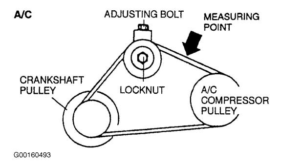
Fig. 23: Identifying Drive Belt Routing & Deflection Check Point (MPV, 3 Of 3) Courtesy of MAZDA MOTORS CORP.
