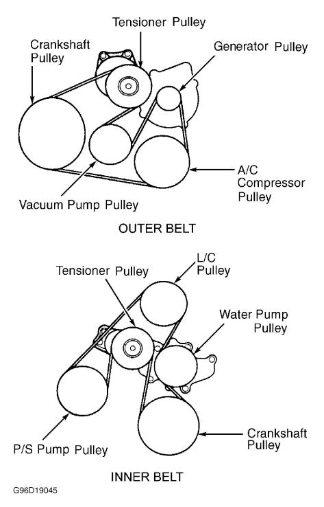
Fig. 18: Identifying Drive Belt Routing (Millenia, 2.3L) Courtesy of FORD MOTOR CO.
