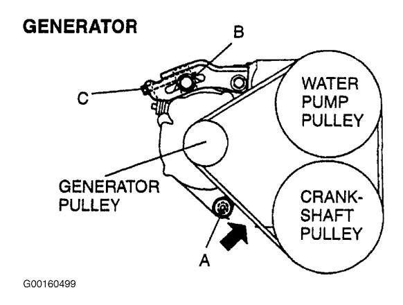
Fig. 12: Adjusting Alternator Belt (Protege) Courtesy of MAZDA MOTORS CORP.
