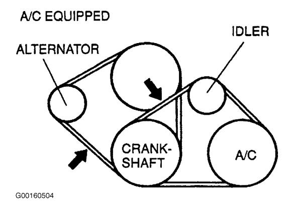
Fig. 26: Identifying Drive Belt Routing & Deflection Check Point (MX-5 Miata, 3 Of 3) Courtesy of MAZDA MOTORS CORP.
