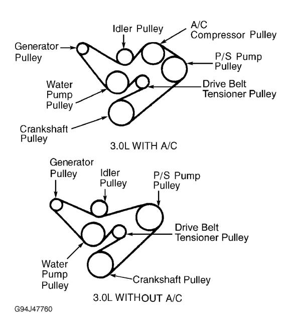
Fig. 16: Identifying Drive Belt Routing (B3000) Courtesy of FORD MOTOR CO.
