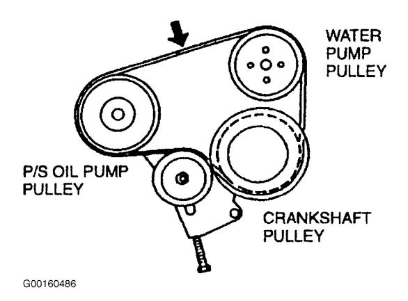
Fig. 20: Identifying Drive Belt Routing & Deflection Check Point (Millenia, 2.5L, 2 Of 2) Courtesy of MAZDA MOTORS CORP.
