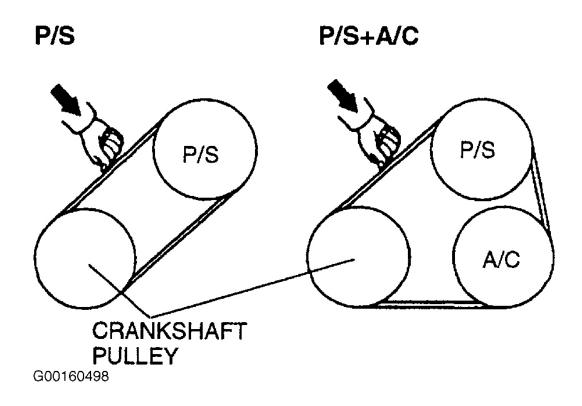
Fig. 28: Identifying Drive Belt Routing & Deflection Check Point (Protege, 2 Of 2) Courtesy of MAZDA MOTORS CORP.
