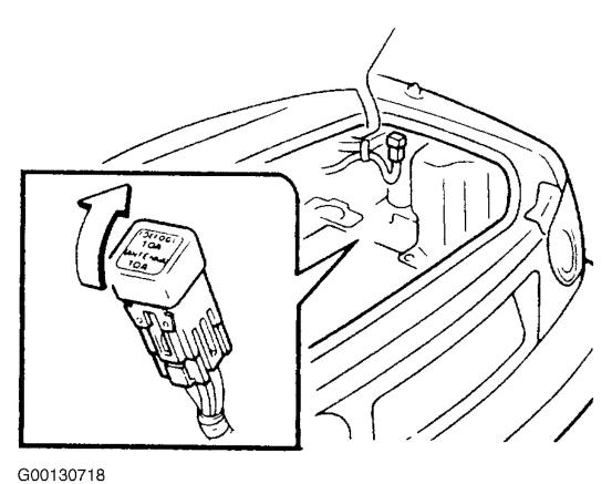
Fig. 7: Locating Trunk Fuse Panel Courtesy of MAZDA MOTORS CORP.
