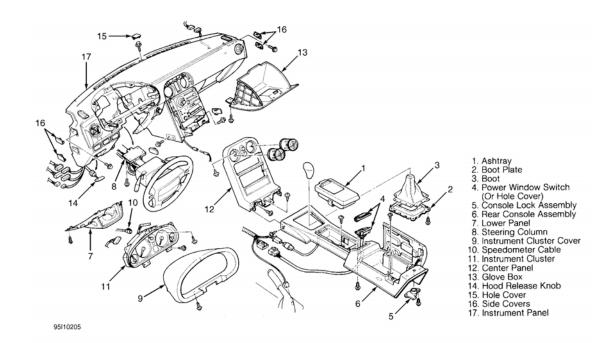
**Fig. 5: Exploded View Of Instrument Panel** Courtesy of MAZDA MOTORS CORP.
