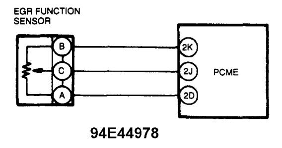
Fig. 14: Trouble Code No. 16 Circuit Diagram (Miata) Courtesy of MAZDA MOTORS CORP.
