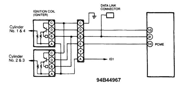
Fig. 4: Trouble Code No. 1 Ignition System Circuit Diagram Courtesy of MAZDA MOTORS CORP.
