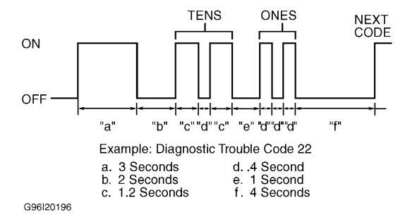
Fig. 2: Reading Diagnostic Trouble Code Output Courtesy of MAZDA MOTORS CORP.
