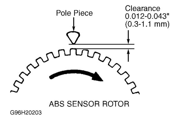
**Fig. 13: Measuring Wheel Speed Sensor Clearance Courtesy of MAZDA MOTORS CORP.**
