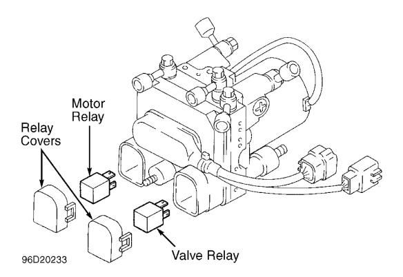
Fig. 14: Locating Valve Relay & Motor Relay Courtesy of MAZDA MOTORS CORP.
