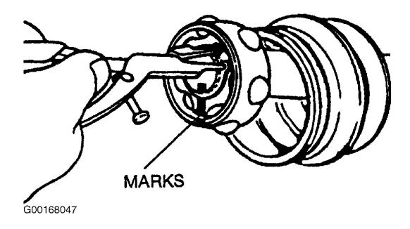
Fig. 7: Removing Snap Ring Courtesy of MAZDA MOTORS CORP.
