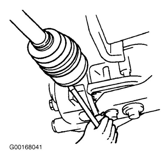
Fig. 2: Prying Out Axle Shaft
