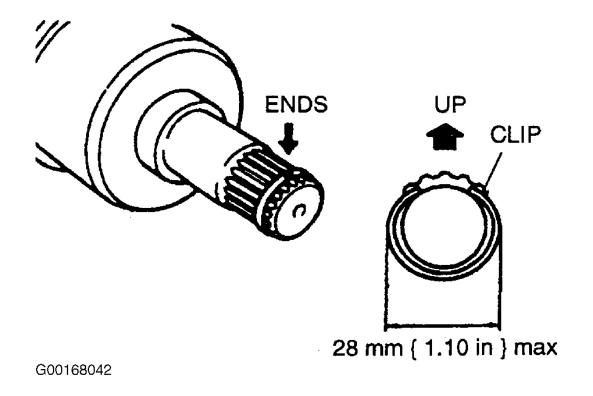
Fig. 3: Measuring Clip Outer Diameter Courtesy of MAZDA MOTORS CORP.
