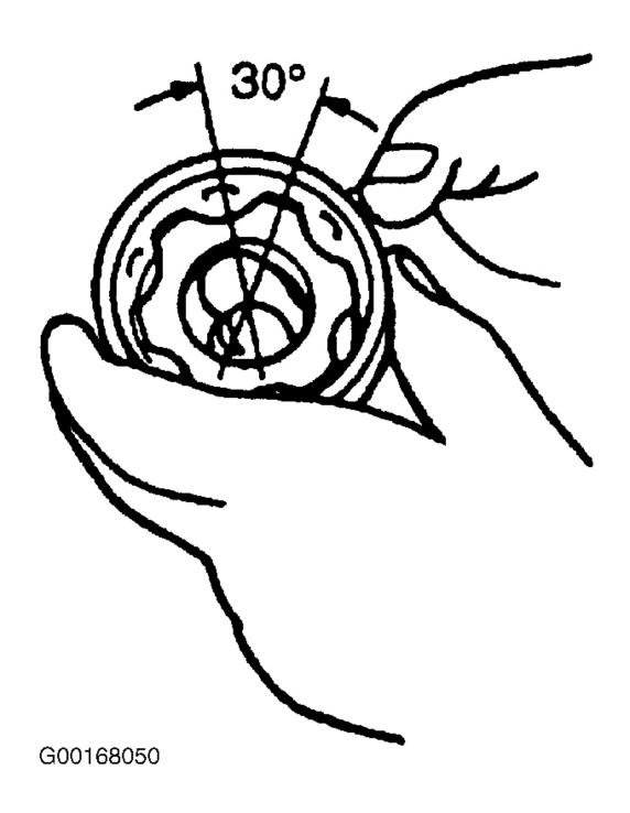
Fig. 9: Separating Inner Ring From Cage Courtesy of MAZDA MOTORS CORP.
