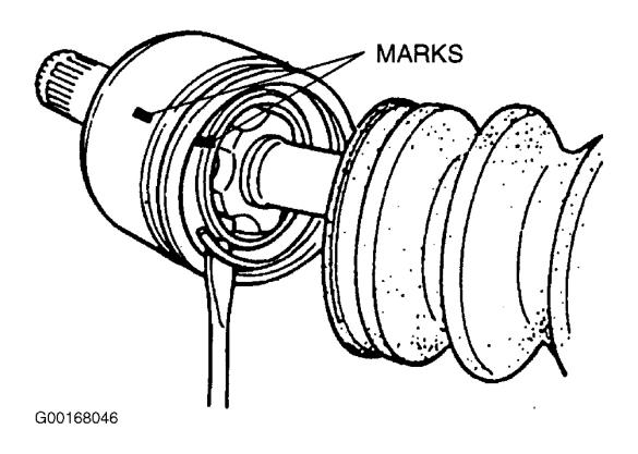
Fig. 6: Marking Axle Shaft & Outer Ring Courtesy of MAZDA MOTORS CORP.
