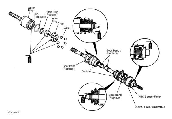
Fig. 11: Exploded View Of Axle Shaft Assembly
