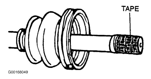
Fig. 10: Removing CV Joint Boot Courtesy of MAZDA MOTORS CORP.
