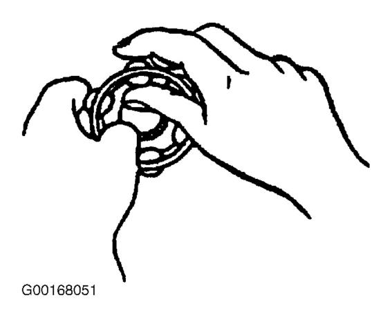
Fig. 8: Removing Balls From Inner Ring Courtesy of MAZDA MOTORS CORP.
