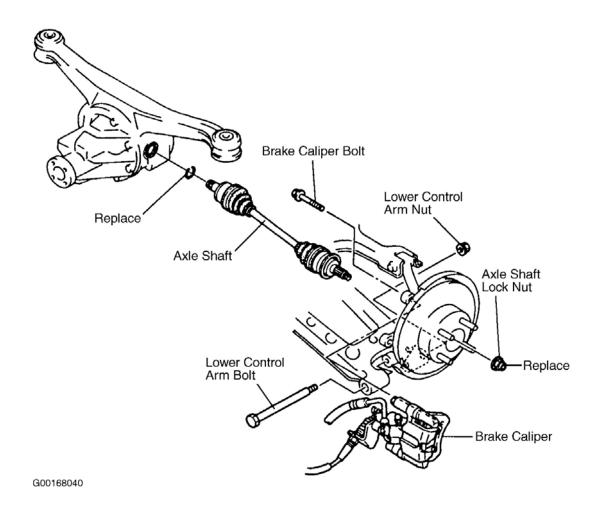
Fig. 1: Removing Axle Shaft Courtesy of MAZDA MOTORS CORP.
