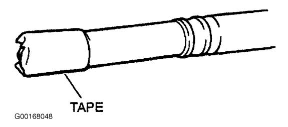
Fig. 12: Installing CV Joint Boot Courtesy of MAZDA MOTORS CORP.
