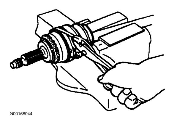
Fig. 15: Installing Boot Band Courtesy of MAZDA MOTORS CORP.
