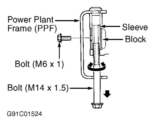
Fig. 6: Removing Reamer Bolt Sleeve (Miata) Courtesy of MAZDA MOTORS CORP.
