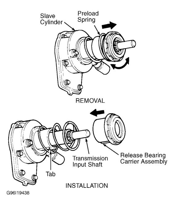
Fig. 8: Servicing Clutch Release Bearing (B2300, B2500, B3000 & B4000) Courtesy of FORD MOTOR CO.
