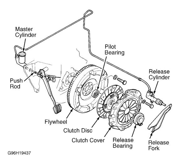
Fig. 7: Exploded View Of Clutch Assembly (Typical) Courtesy of MAZDA MOTORS CORP.
