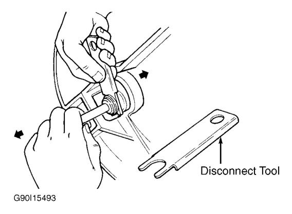
Fig. 2: Removing Hydraulic Line (B2300, B2500, B3000 & B4000) Courtesy of MAZDA MOTORS CORP.
