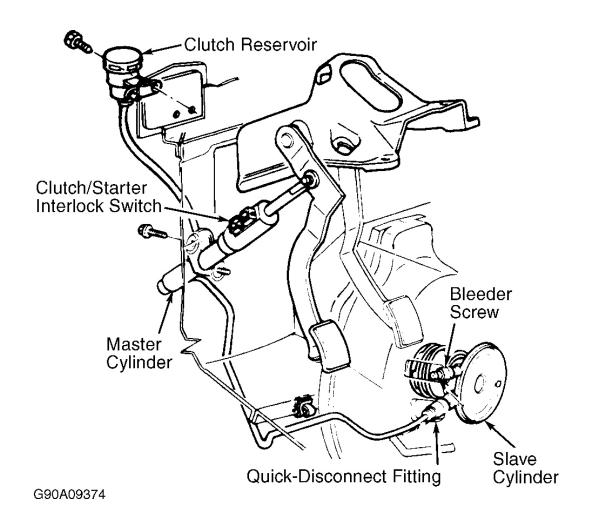
Fig. 9: Removing Clutch/Starter Interlock Switch (B2300, B2500, B3000 & B4000) Courtesy of FORD MOTOR CO.
