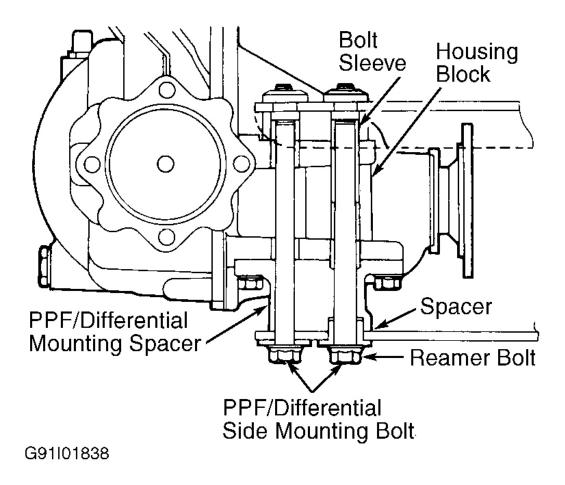
Fig. 5: Installing & Removing Power Plant Frame (Miata) Courtesy of MAZDA MOTORS CORP.
