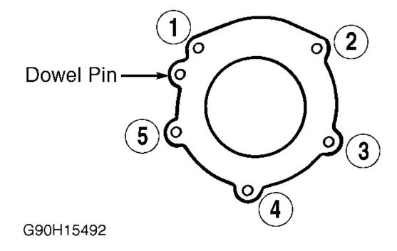
Fig. 3: Tightening Transfer Case Bolts (B2300, B2500, B3000 & B4000) Courtesy of MAZDA MOTORS CORP.
