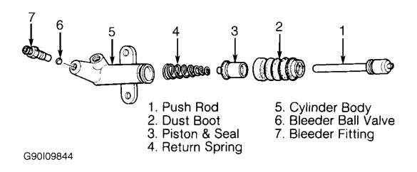
Fig. 11: Exploded View Of Clutch Release Cylinder (Miata) Courtesy of MAZDA MOTORS CORP.
