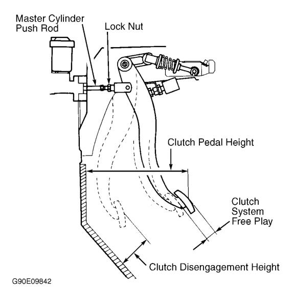
Fig. 1: Adjusting Clutch Pedal (Miata) Courtesy of MAZDA MOTORS CORP.
