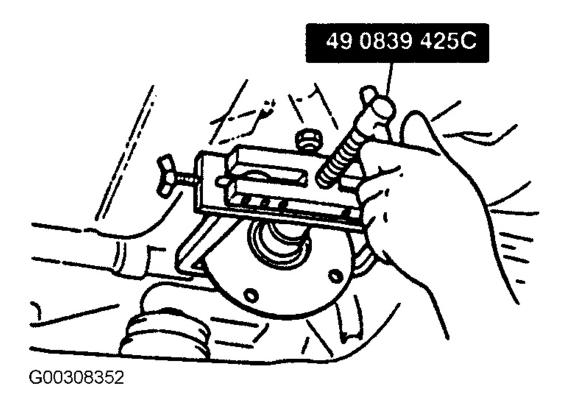
Fig. 3: Removing Companion Flange (MPV) Courtesy of MAZDA MOTORS CORP.
