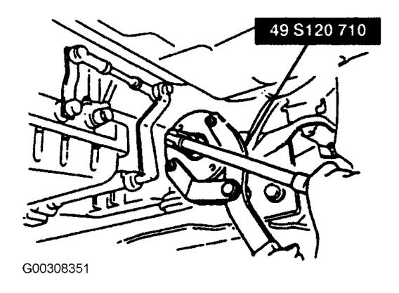
Fig. 2: Holding Companion Flange (MPV) Courtesy of MAZDA MOTORS CORP.
