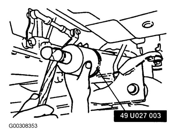
Fig. 4: Installing Oil Seal (MPV)
