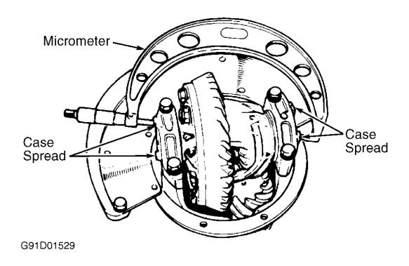
Fig. 13: Measuring Carrier Case Spread Courtesy of MAZDA MOTORS CORP.
