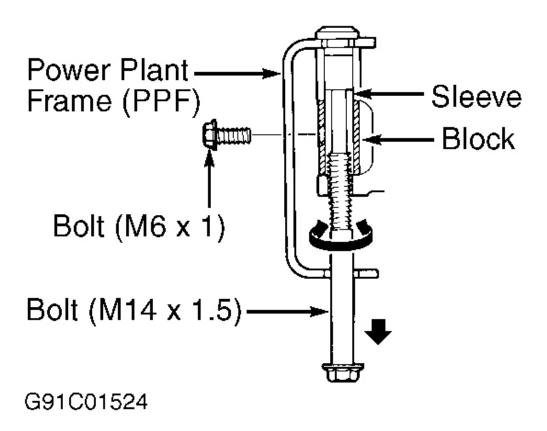
Fig. 9: Removing Reamer Bolt Sleeve (Miata) Courtesy of MAZDA MOTORS CORP.
