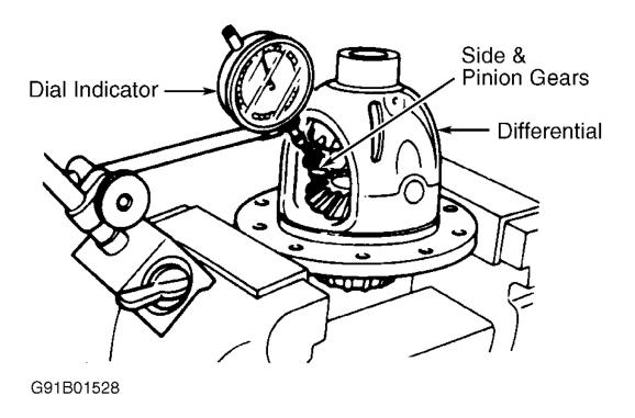
Fig. 11: Measuring Side Gear & Pinion Gear Backlash Courtesy of MAZDA MOTORS CORP.
