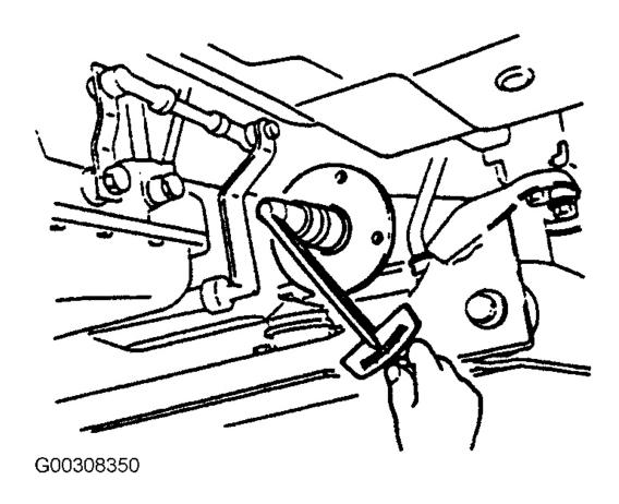
Fig. 1: Measuring Rotation Starting Torque (MPV) Courtesy of MAZDA MOTORS CORP.
