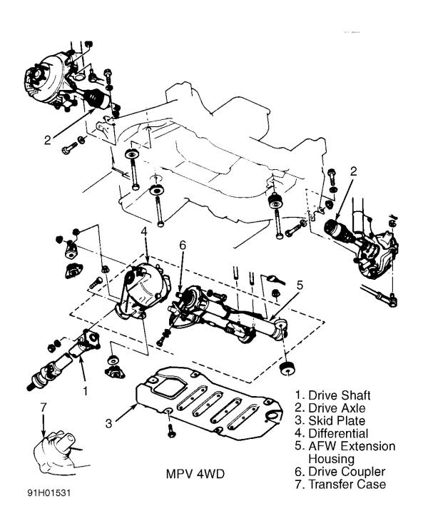
Fig. 6: Removing & Installing Front Differential (MPV 4WD) Courtesy of MAZDA MOTORS CORP.
