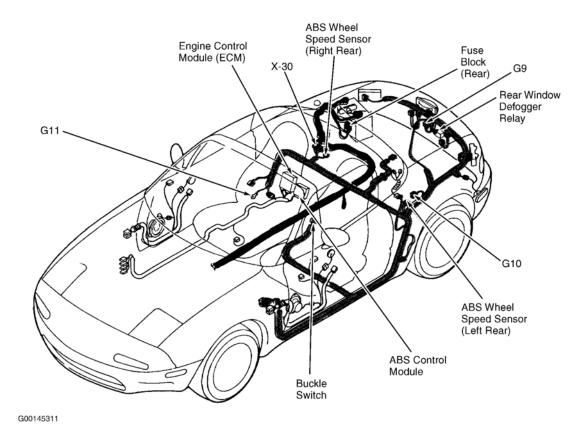
Fig. 3: Left Side Of Vehicle
