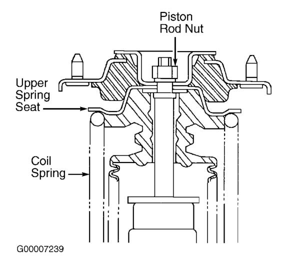
Fig. 2: Cross-Sectional View Of Upper Coil Over Shock Assembly (1997) Courtesy of MAZDA MOTORS CORP.
