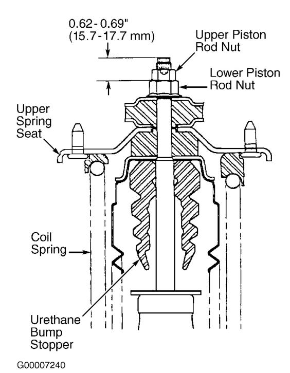
Fig. 3: Cross-Sectional View Of Upper Coil Over Shock Assembly (1999-2000) Courtesy of MAZDA MOTORS CORP.
