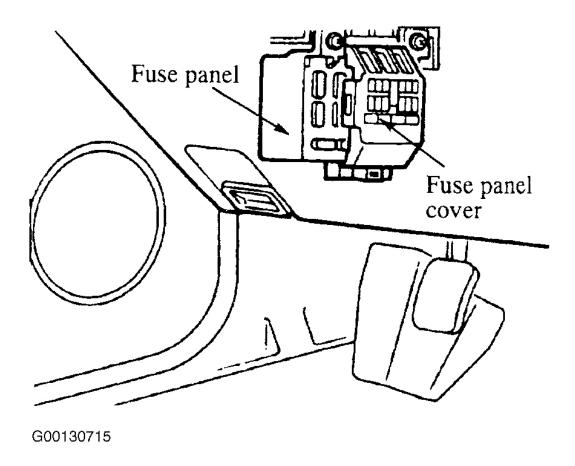
Fig. 4: Locating Fuse Block Courtesy of MAZDA MOTORS CORP.
