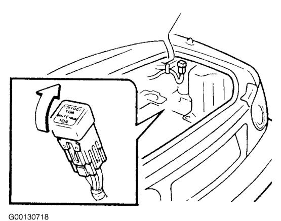
Fig. 7: Locating Trunk Fuse Box Courtesy of MAZDA MOTORS CORP.
