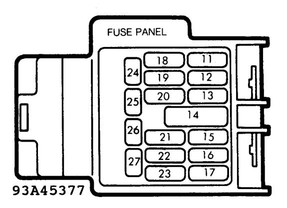
Fig. 5: Interior Fuse Panel Identification Courtesy of MAZDA MOTOR OF AMERICA, INC.
