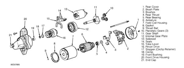
**Fig. 4: Exploded View Of Coaxial Planetary Gear Type Starter** Courtesy of MAZDA MOTORS CORP.
