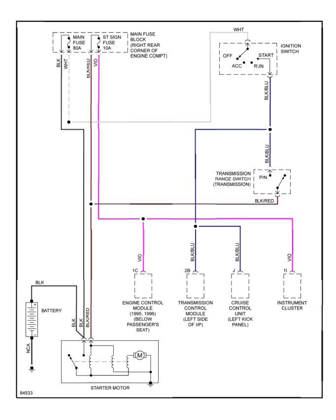
STARTER - REDUCTION GEAR 1997 STARTING & CHARGING SYSTEMS Mazda - Starters - Reduction Gear
