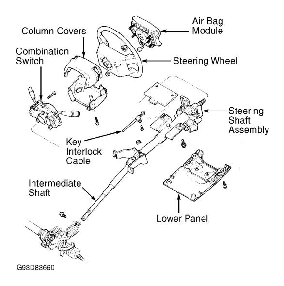
Fig. 5: Exploded View Of Steering Column (Miata) Courtesy of MAZDA MOTORS CORP.
