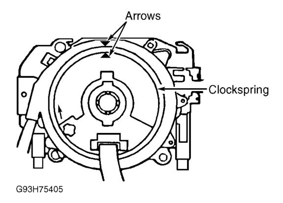
Fig. 4: Centering Clockspring Courtesy of MAZDA MOTORS CORP.
