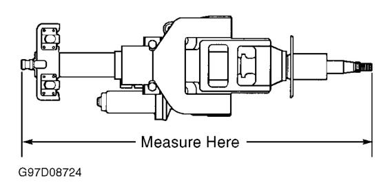
Fig. 13: Measuring Steering Shaft Dimensions (Millenia) Courtesy of MAZDA MOTORS CORP.
