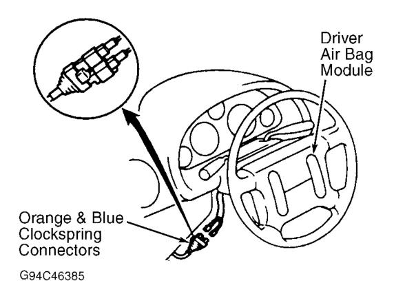
Fig. 1: Disconnecting Clockspring Connectors (Typical) Courtesy of MAZDA MOTORS CORP.
