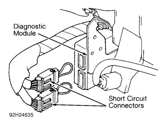
Fig. 3: Connecting Short Circuit Connectors (Typical) Courtesy of MAZDA MOTORS CORP.
