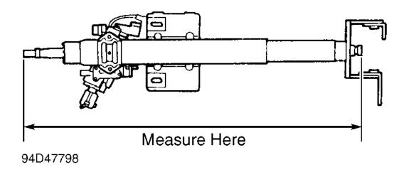
Fig. 18: Measuring Steering Shaft Dimensions (929) Courtesy of MAZDA MOTORS CORP.
