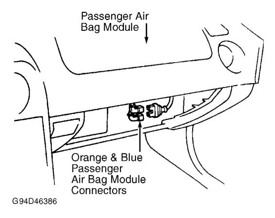
Fig. 2: Disconnecting Passenger Air Bag Module Connectors (Typical) Courtesy of MAZDA MOTORS CORP.
