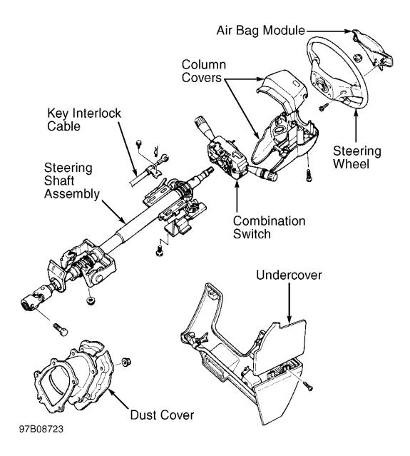
Fig. 8: Exploded View Of Steering Column (MX-3 & Protege) Courtesy of MAZDA MOTORS CORP.
