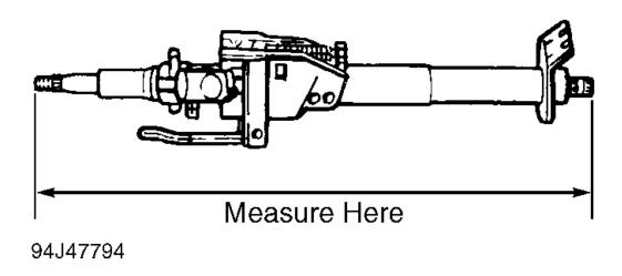
Fig. 14: Measuring Steering Shaft Dimensions (MPV) Courtesy of MAZDA MOTORS CORP.
