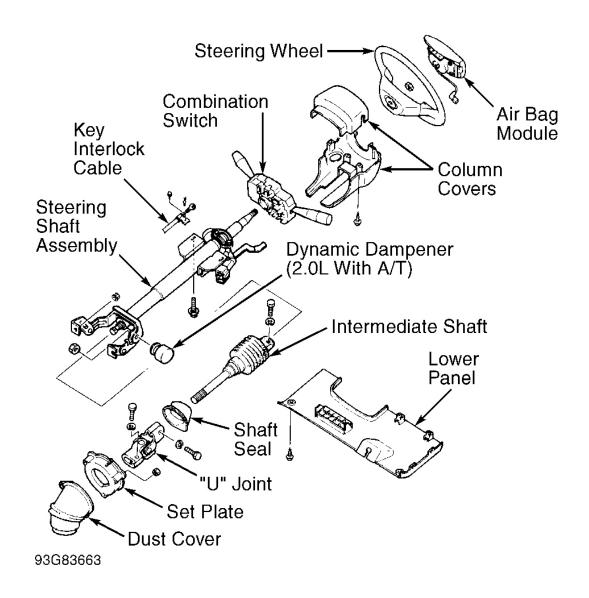
Fig. 9: Exploded View Of Steering Column (MX-6 & 626) Courtesy of MAZDA MOTORS CORP.
