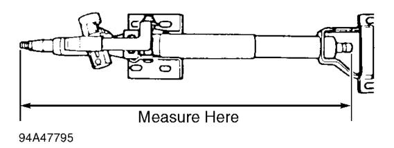
Fig. 15: Measuring Steering Shaft Dimensions (MX-3, Protege & 323) Courtesy of MAZDA MOTORS CORP.
