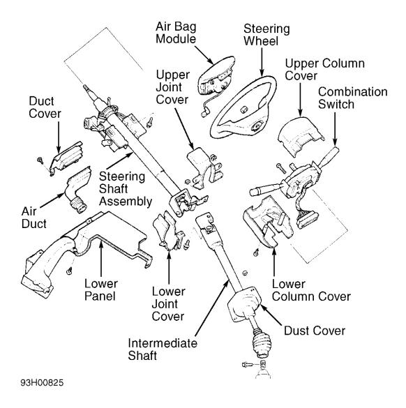
Fig. 11: Exploded View Of Steering Column (929) Courtesy of MAZDA MOTORS CORP.
