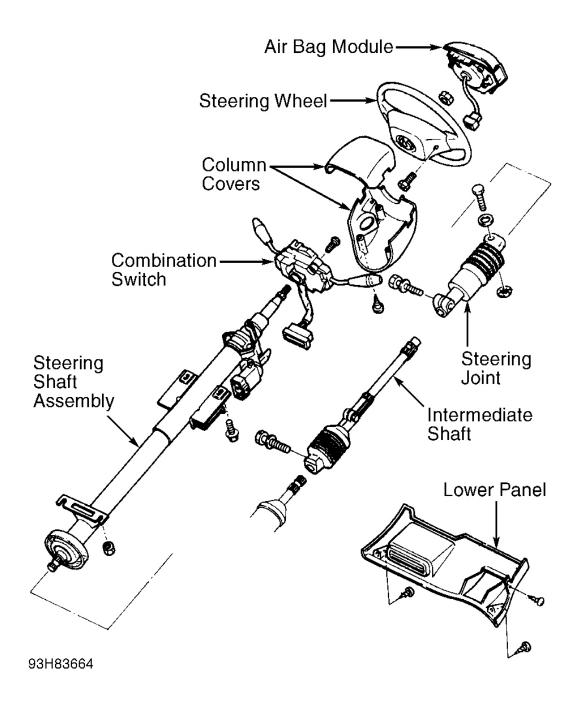
Fig. 10: Exploded View Of Steering Column (RX7) Courtesy of MAZDA MOTORS CORP.
