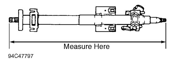
Fig. 17: Measuring Steering Shaft Dimensions (RX7) Courtesy of MAZDA MOTORS CORP.
