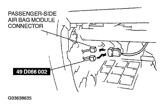
Fig. 30: Connecting Adapter Harness To Passenger-Side Air Bag Module Courtesy of MAZDA MOTORS CORP.
