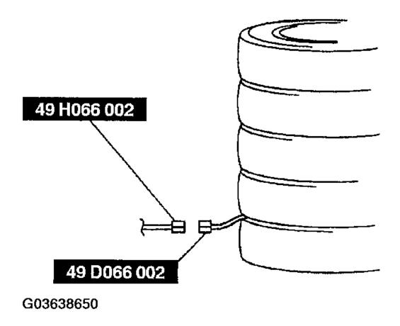
Fig. 45: Connecting Deployment Tool To Adapter Harness Courtesy of MAZDA MOTORS CORP.
