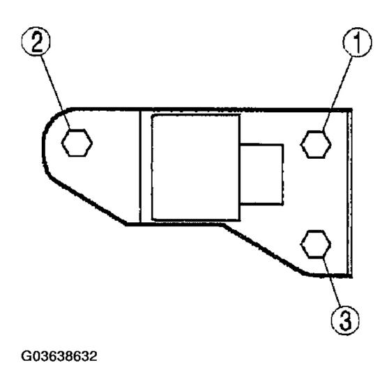
Fig. 27: Tightening Crush Zone Sensor Bolts In Order Courtesy of MAZDA MOTORS CORP.
