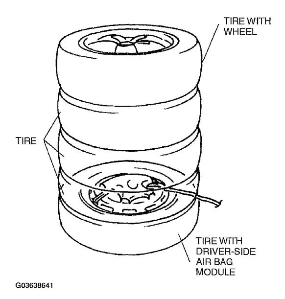
Fig. 36: Stacking Tires - For Driver-Side Air Bag Module Courtesy of MAZDA MOTORS CORP.
