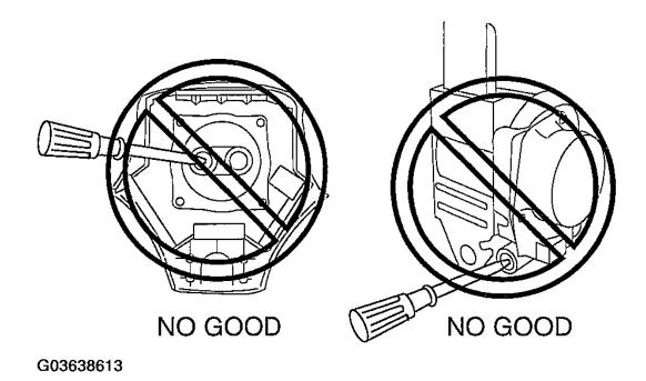
Fig. 8: Warning Against Screwdriver Insertion Courtesy of MAZDA MOTORS CORP.
