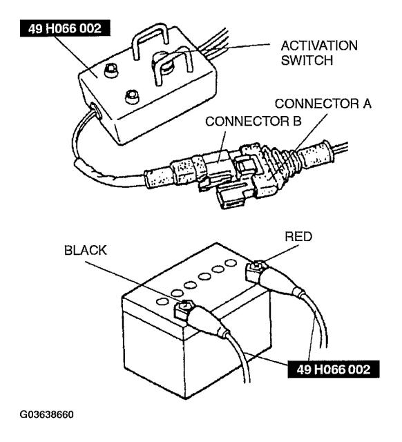
Fig. 55: Inspecting Deployment Tool Courtesy of MAZDA MOTORS CORP.
