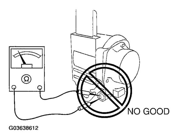
Fig. 7: Identifying Improper Method For Inspecting Pre-Tensioner Seat Belt Courtesy of MAZDA MOTORS CORP.
