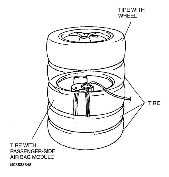
Fig. 43: Stacking Tires - For Passenger-Side Air Bag Module Courtesy of MAZDA MOTORS CORP.
