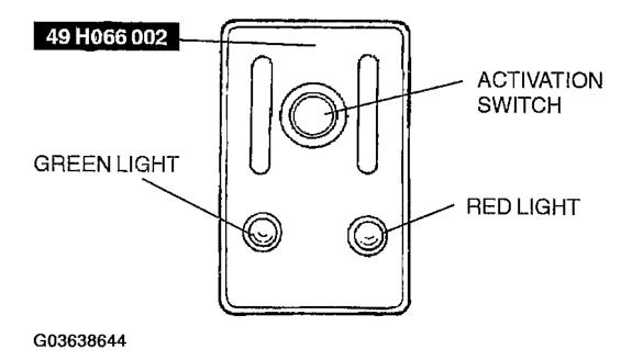
Fig. 39: Identifying Deployment Tool Courtesy of MAZDA MOTORS CORP.
