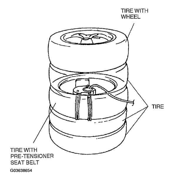
Fig. 49: Stacking Tires - For Pre-Tensioner Seat Belt Courtesy of MAZDA MOTORS CORP.
