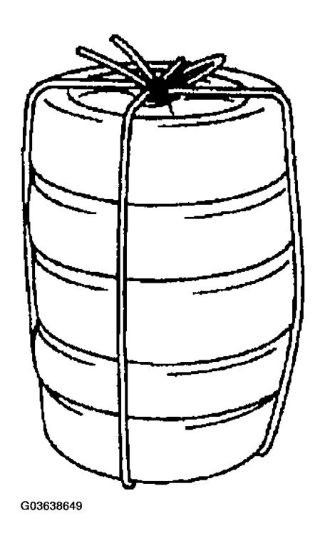
Fig. 44: Tying Tires Together With Wire Courtesy of MAZDA MOTORS CORP.
