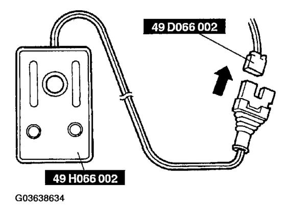
Fig. 29: Connecting Deployment Tool To Adapter Harness Courtesy of MAZDA MOTORS CORP.
