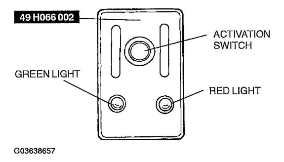
Fig. 52: Identifying Deployment Tool Courtesy of MAZDA MOTORS CORP.
