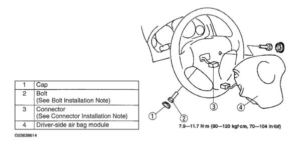
Fig. 9: Removing Driver-Side Air Bag Module Courtesy of MAZDA MOTORS CORP.
