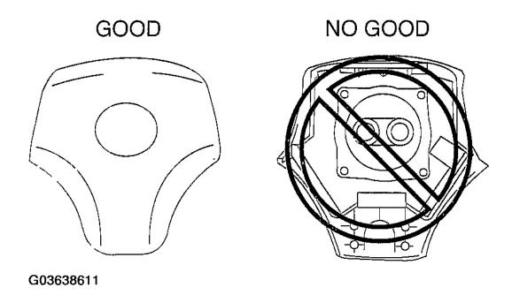
Fig. 6: Identifying Proper Air Bag Module Facing Courtesy of MAZDA MOTORS CORP.
