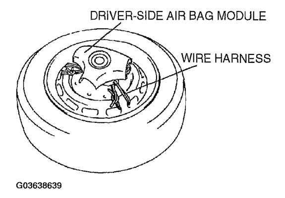
Fig. 34: Placing Driver-Side Air Bag Module On Center Of Wheel With Module Facing Up Courtesy of MAZDA MOTORS CORP.
