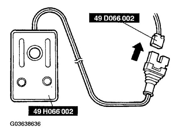
Fig. 31: Connecting Deployment Tool To Adapter Harness Courtesy of MAZDA MOTORS CORP.
