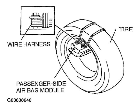
Fig. 41: Tying Passenger-Side Air Bag Module To Tire Courtesy of MAZDA MOTORS CORP.
