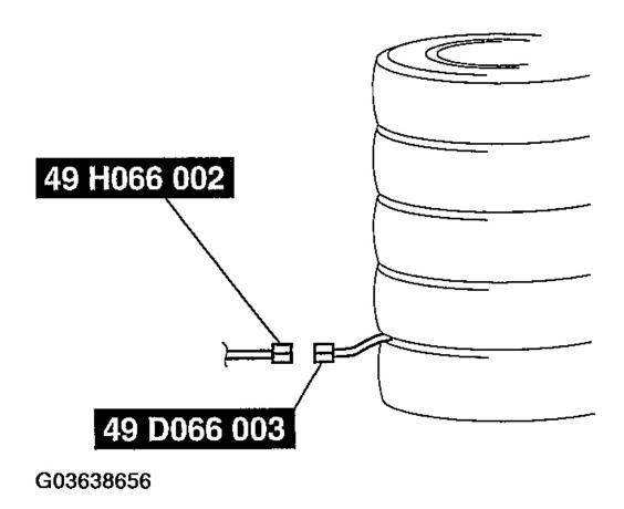
Fig. 51: Connecting Deployment Tool To Adapter Harness Courtesy of MAZDA MOTORS CORP.
