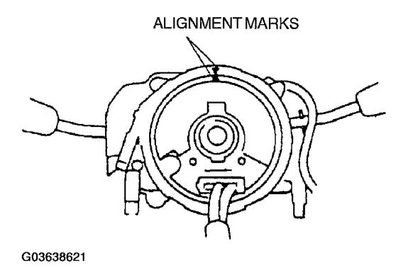
Fig. 16: Aligning Mark On Clock Spring With Mark On Outer Housing Courtesy of MAZDA MOTORS CORP.
