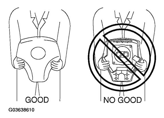
Fig. 5: Identifying Proper Air Bad Module Carrying Method Courtesy of MAZDA MOTORS CORP.
