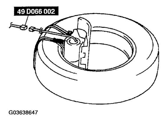
Fig. 42: Connecting Adapter Harness To Passenger-Side Air Bag Module Courtesy of MAZDA MOTORS CORP.
