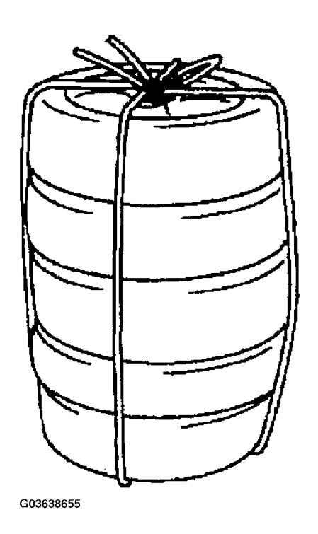
Fig. 50: Tying Tires Together With Wire Courtesy of MAZDA MOTORS CORP.
