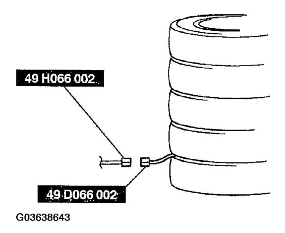
Fig. 38: Connecting Deployment Tool To Adapter Harness Courtesy of MAZDA MOTORS CORP.
