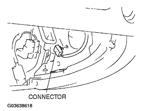
Fig. 13: Installing Connector Courtesy of MAZDA MOTORS CORP.
