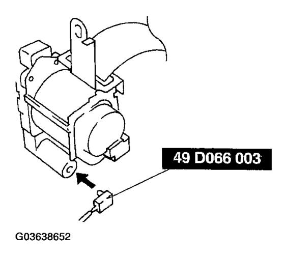
Fig. 47: Connecting Adapter Harness To Pre-Tensioner Seat Belt Courtesy of MAZDA MOTORS CORP.
