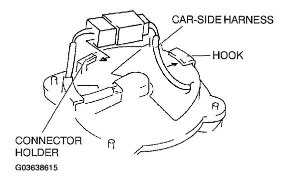
Fig. 10: Installing Connector Courtesy of MAZDA MOTORS CORP.
