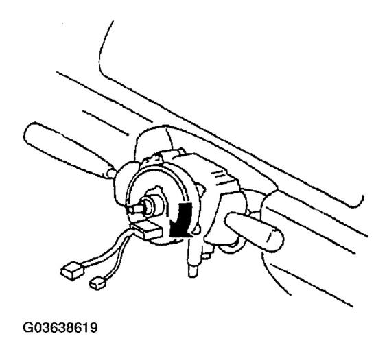
Fig. 14: Turning Clock Spring Clockwise Until Stops Courtesy of MAZDA MOTORS CORP.
