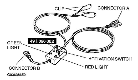
Fig. 54: Identifying Deployment Tool Components Courtesy of MAZDA MOTORS CORP.
