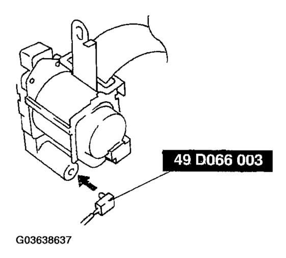
Fig. 32: Connecting Adapter Harness To Pre-Tensioner Seat Belt Courtesy of MAZDA MOTORS CORP.
