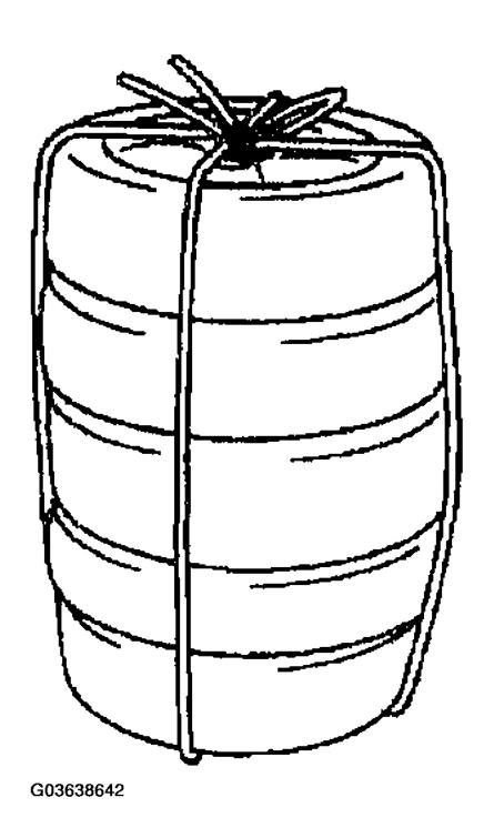
Fig. 37: Tying Tires Together With Wire Courtesy of MAZDA MOTORS CORP.
