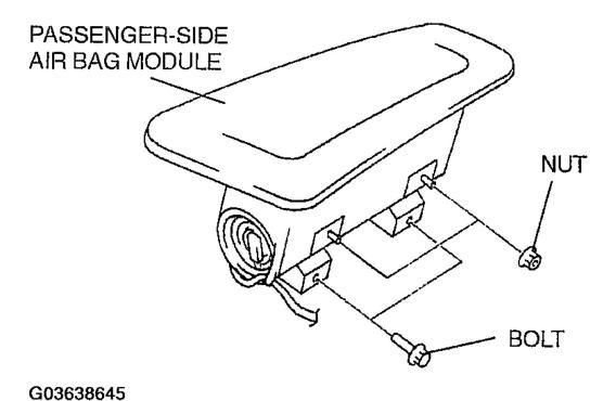
Fig. 40: Installing Passenger-Side Air Bag Module Courtesy of MAZDA MOTORS CORP.
