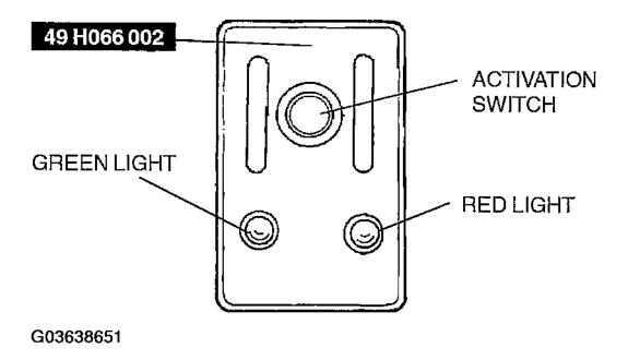
Fig. 46: Identifying Deployment Tool Courtesy of MAZDA MOTORS CORP.
