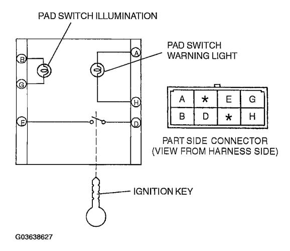
Fig. 22: Identifying Passenger Air Bag Terminal Connectors Courtesy of MAZDA MOTORS CORP.
