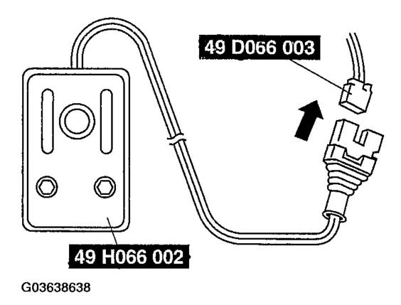
Fig. 33: Connecting Deployment Tool To Adapter Harness Courtesy of MAZDA MOTORS CORP.
