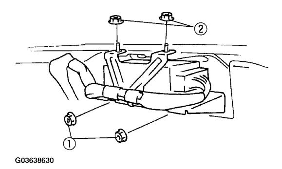
Fig. 25: Tightening SAS Control Module Nuts In Order Courtesy of MAZDA MOTORS CORP.
