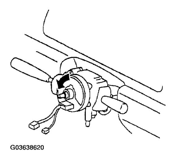
Fig. 15: Turning Clock Spring Counterclockwise Courtesy of MAZDA MOTORS CORP.
