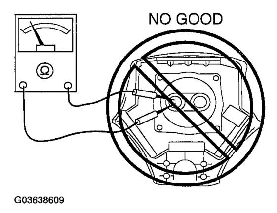
Fig. 4: Inspecting Air Bag Module Incorrectly Courtesy of MAZDA MOTORS CORP.
