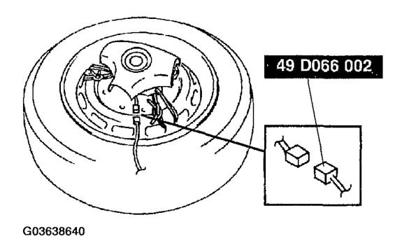
Fig. 35: Connecting Adapter Harness To Driver-Side Air Bag Module Courtesy of MAZDA MOTORS CORP.
