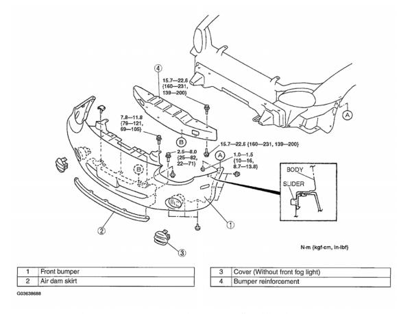
Fig. 11: Removing Front Bumper - With Torque Specifications Courtesy of MAZDA MOTORS CORP.
