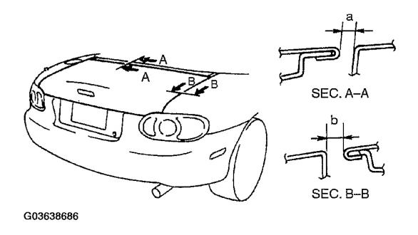
Fig. 9: Adjusting Trunk Lid Courtesy of MAZDA MOTORS CORP.
