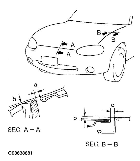
Fig. 4: Adjusting Hood Courtesy of MAZDA MOTORS CORP.
