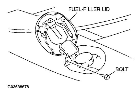
Fig. 1: Removing Fuel-Filler Lid Courtesy of MAZDA MOTORS CORP.
