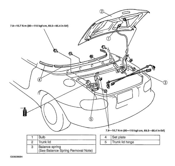
Fig. 7: Removing Trunk Lid Courtesy of MAZDA MOTORS CORP.
