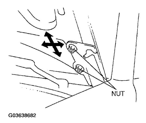
Fig. 5: Adjusting Hood Gap Courtesy of MAZDA MOTORS CORP.
