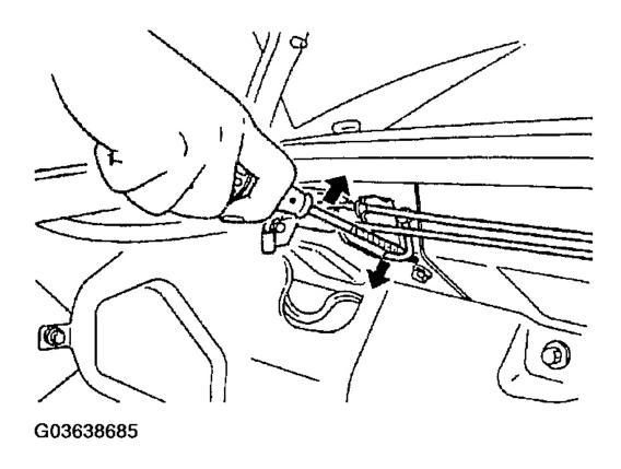
Fig. 8: Removing Balance Spring Courtesy of MAZDA MOTORS CORP.
