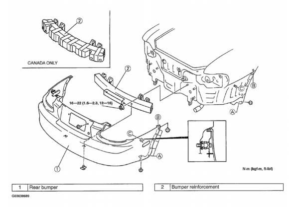
Fig. 12: Removing Rear Bumper - With Torque Specifications Courtesy of MAZDA MOTORS CORP.
