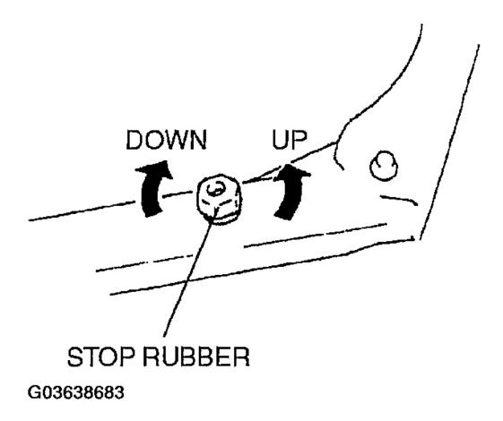
Fig. 6: Adjusting Hood Height Courtesy of MAZDA MOTORS CORP.
