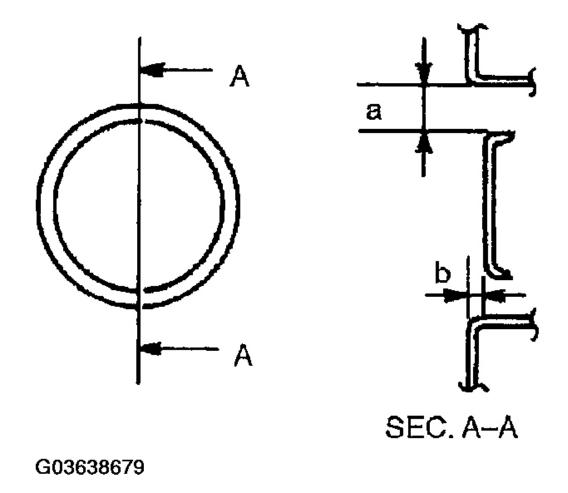
Fig. 2: Adjusting Fuel Filler Lid Courtesy of MAZDA MOTORS CORP.
