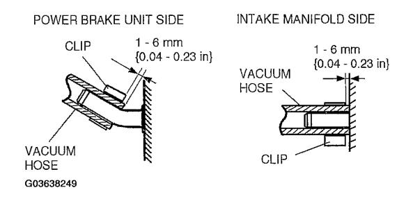
**Fig. 25: Installing Vacuum Hose To Power Brake Unit And Intake Manifold Courtesy of MAZDA MOTORS CORP.**
