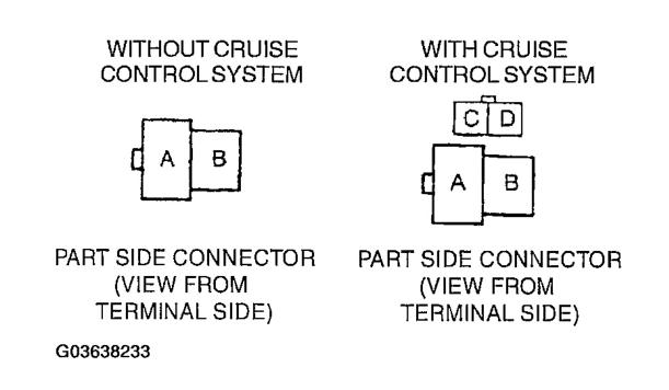
**Fig. 9: Identifying Brake Switch Connectors Courtesy of MAZDA MOTORS CORP.**
