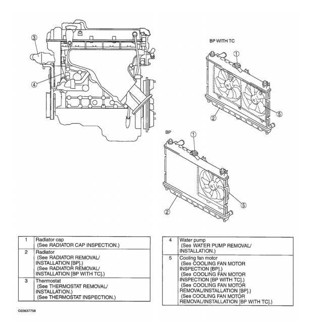
Fig. 1: Identifying Cooling System Location Index Courtesy of MAZDA MOTORS CORP.
