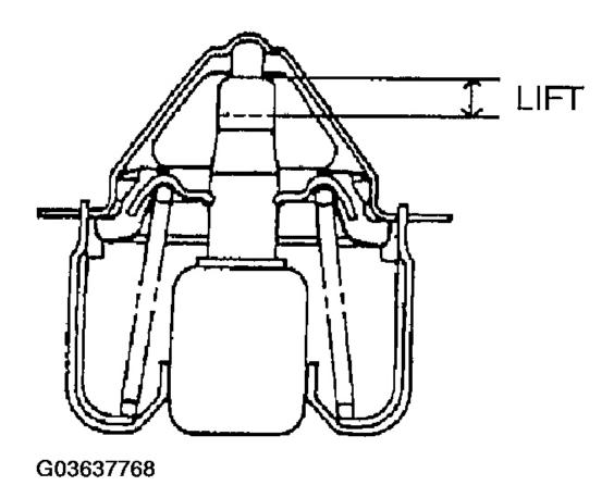
Fig. 11: Identifying Full-Open Lift Courtesy of MAZDA MOTORS CORP.
