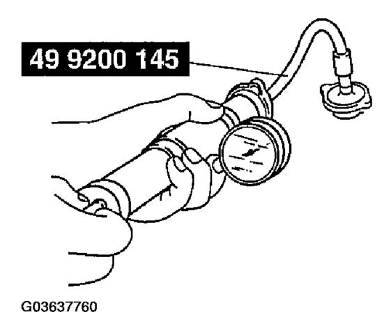
Fig. 3: Connecting Radiator Cap Tester And SST To Radiator Filler Neck Courtesy of MAZDA MOTORS CORP.
