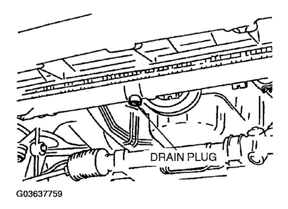
Fig. 2: Removing Radiator Cap And Radiator Drain Plug Courtesy of MAZDA MOTORS CORP.
