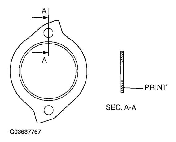
Fig. 10: Installing Gasket With Seal Print Side Facing Cylinder Head Courtesy of MAZDA MOTORS CORP.
