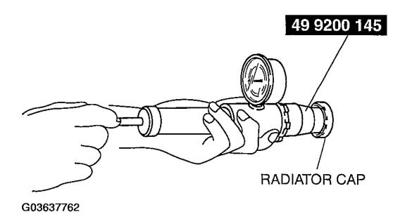
Fig. 5: Attaching Radiator Cap To Radiator Cap Tester With SST Courtesy of MAZDA MOTORS CORP.
