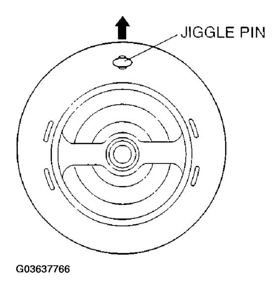
Fig. 9: Installing Thermostat Into Cylinder Head With Jiggle Pin At Top Courtesy of MAZDA MOTORS CORP.
