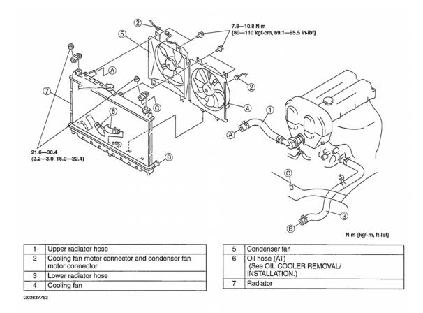
Fig. 6: Exploded View Of Radiator & Torque Specifications Courtesy of MAZDA MOTORS CORP.
