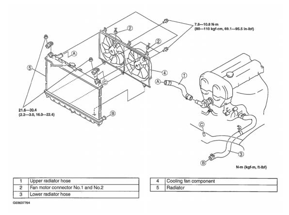
Fig. 7: Exploded View Of Radiator With Torque Specifications Courtesy of MAZDA MOTORS CORP.
