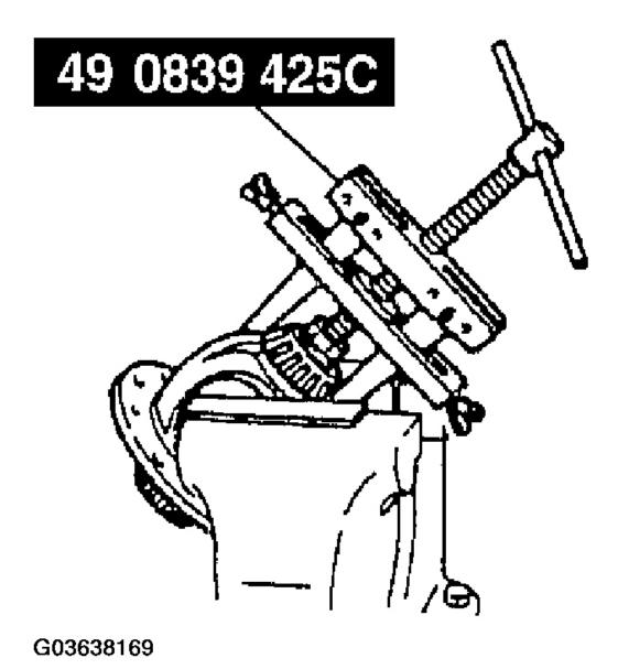
Fig. 24: Removing Bearing Inner Races (Side Bearing) From Gear Case Using SST Courtesy of MAZDA MOTORS CORP.
