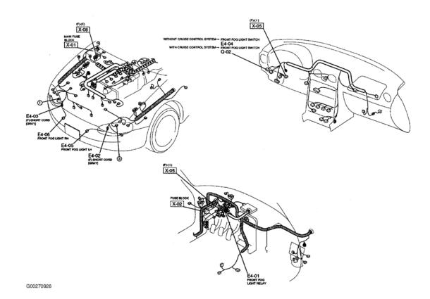
**Fig. 26: Fog Lights** Courtesy of MAZDA MOTORS CORP.
