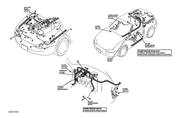
**Fig. 10: Power Windows** Courtesy of MAZDA MOTORS CORP.
