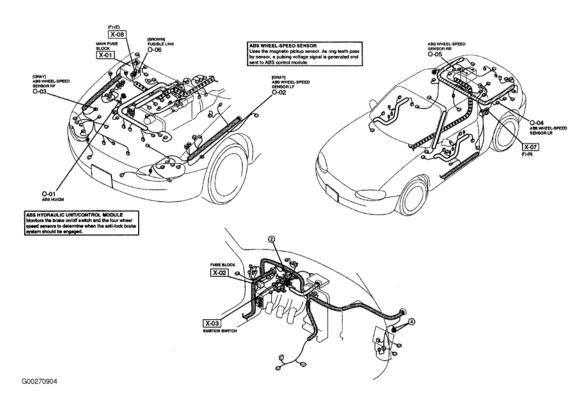
Fig. 7: Anti-Lock Brake System Courtesy of MAZDA MOTORS CORP.
