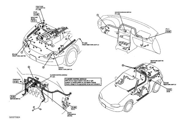
**Fig. 24: Turn Signal & Hazard Lights** Courtesy of MAZDA MOTORS CORP.
