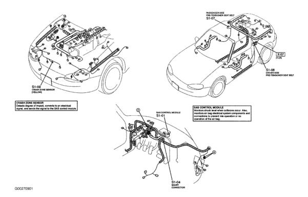
**Fig. 5: Air Bag System** Courtesy of MAZDA MOTORS CORP.
