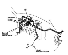
**Fig. 19: Shift-Lock** Courtesy of MAZDA MOTORS CORP.
