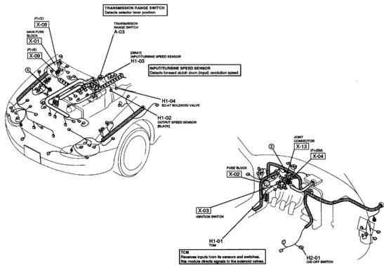
Fig. 20: EC-AT Control Courtesy of MAZDA MOTORS CORP.
