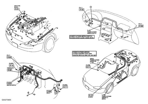
Fig. 8: Power Mirrors Courtesy of MAZDA MOTORS CORP.
