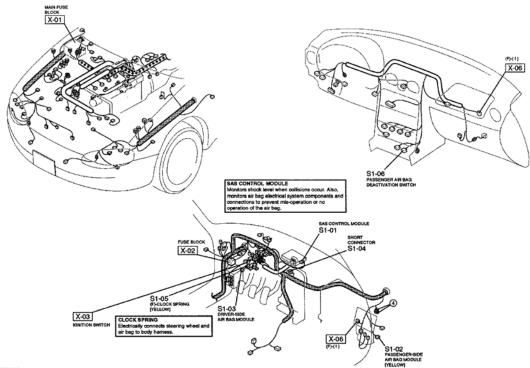
**Fig. 4: Air Bag System** Courtesy of MAZDA MOTORS CORP.
