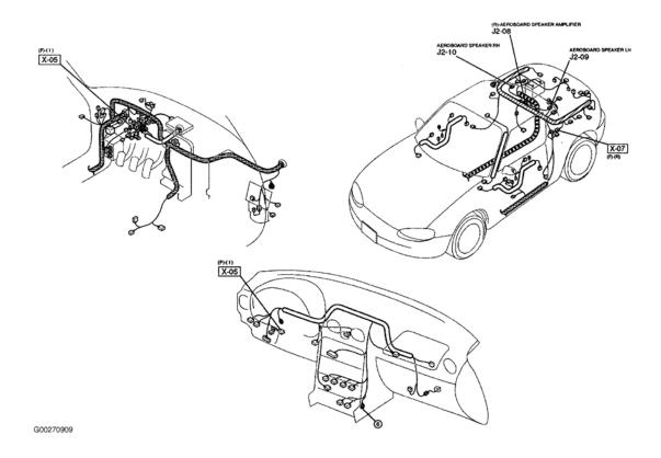
Fig. 14: Audio (W/Bose) Courtesy of MAZDA MOTORS CORP.
