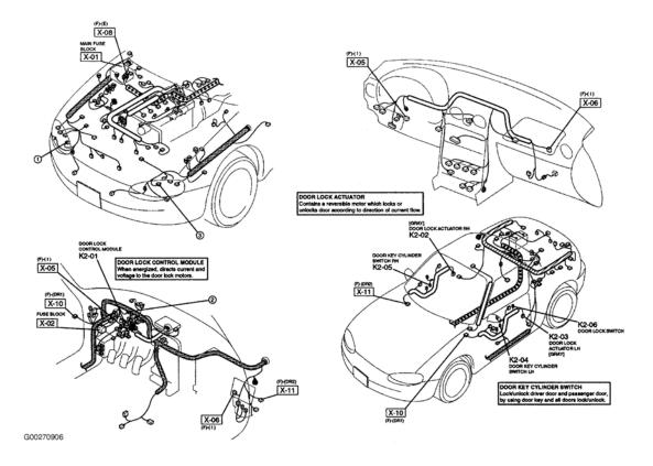
**Fig. 9: Door Locks** Courtesy of MAZDA MOTORS CORP.
