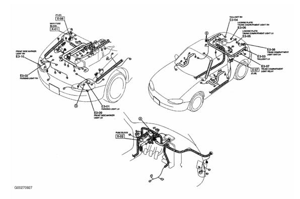
Fig. 27: Front Side Marker, License, Trunk & Parking Lights Courtesy of MAZDA MOTORS CORP.
