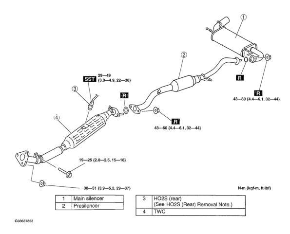
Fig. 3: Identifying Components Of Exhaust System & Torque Specifications Courtesy of MAZDA MOTORS CORP.
