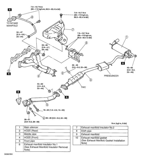
Fig. 1: Identifying Components Of Exhaust System & Torque Specifications Courtesy of MAZDA MOTORS CORP.
