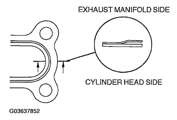
Fig. 2: Identifying Exhaust Manifold Side Courtesy of MAZDA MOTORS CORP.
