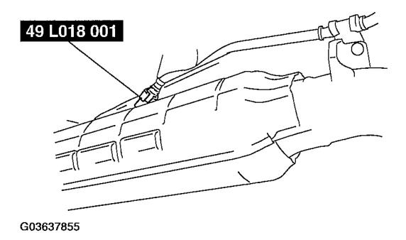
Fig. 5: Disconnecting HO2S (Rear) Connector Courtesy of MAZDA MOTORS CORP.
