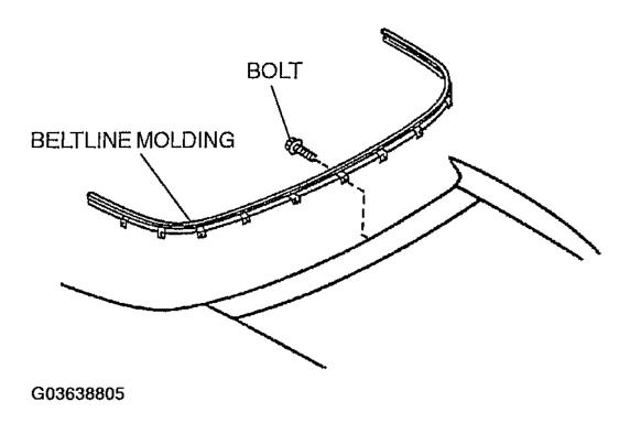
Fig. 2: Removing Beltline Molding Courtesy of MAZDA MOTORS CORP.
