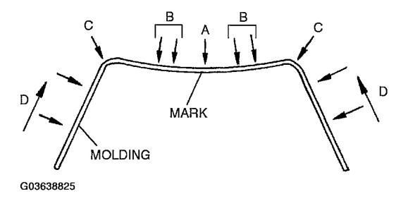
Fig. 22: Identifying Molding Courtesy of MAZDA MOTORS CORP.
