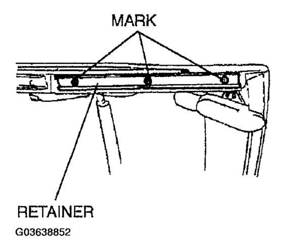
Fig. 49: Marking Around Retainer Installation Screws Courtesy of MAZDA MOTORS CORP.
