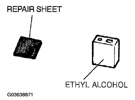
Fig. 68: Degreasing Repair Sheet Using Ethyl Alcohol Courtesy of MAZDA MOTORS CORP.
