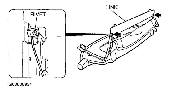
Fig. 31: Removing Rivets From Link Courtesy of MAZDA MOTORS CORP.
