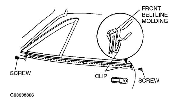
Fig. 3: Removing Front Beltline Molding Courtesy of MAZDA MOTORS CORP.
