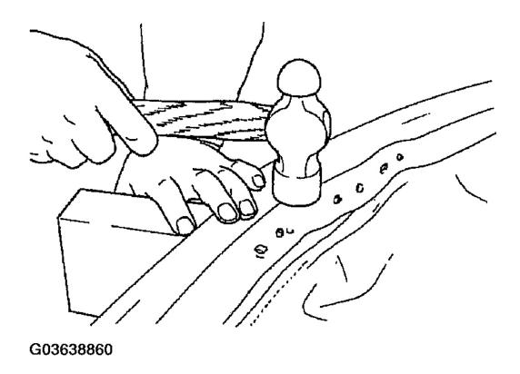
Fig. 57: Flattening Stem Using Hammer Courtesy of MAZDA MOTORS CORP.
