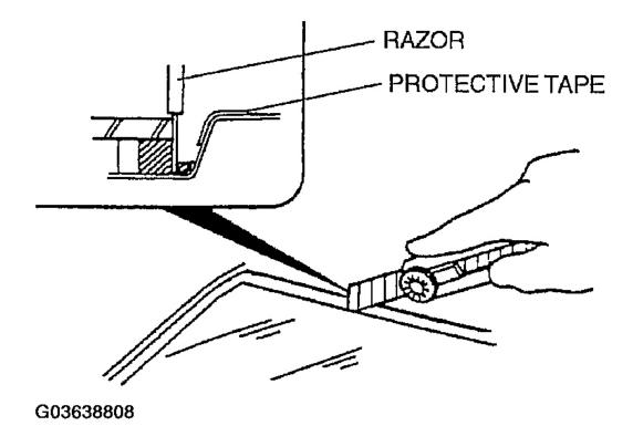
Fig. 5: Cutting Sealant Using Razor Courtesy of MAZDA MOTORS CORP.
