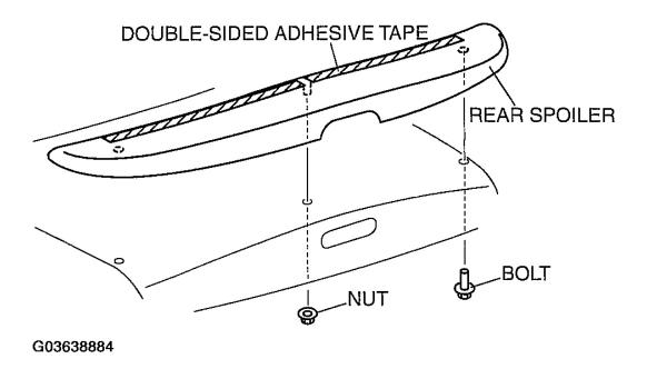
Fig. 81: Removing Rear Spoiler (BP With TC) Courtesy of MAZDA MOTORS CORP.
