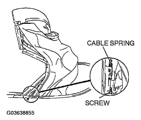
Fig. 52: Identifying Cable Spring And Screw Courtesy of MAZDA MOTORS CORP.
