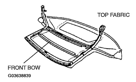
Fig. 36: Installing Top Fabric To Front Bow Courtesy of MAZDA MOTORS CORP.
