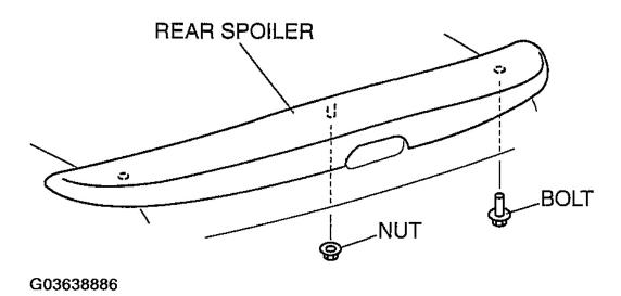
Fig. 83: Installing Rear Spoiler (BP With TC) Courtesy of MAZDA MOTORS CORP.
