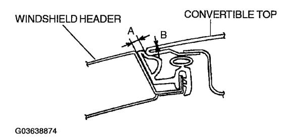
Fig. 71: Adjusting Detachable Hardtop Courtesy of MAZDA MOTORS CORP.
