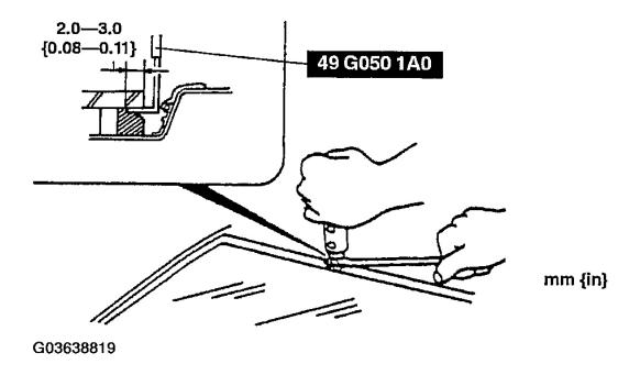
Fig. 16: Cutting Sealant Near Glass Courtesy of MAZDA MOTORS CORP.
