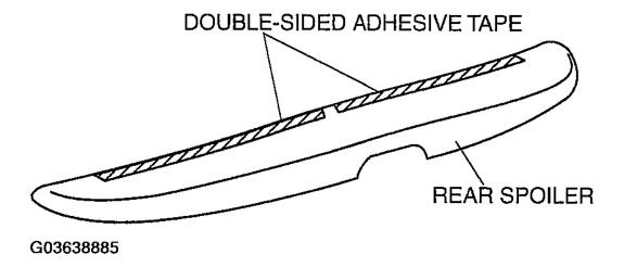
Fig. 82: Affixing Double-Sided Adhesive Tape To Rear Spoiler Courtesy of MAZDA MOTORS CORP.
