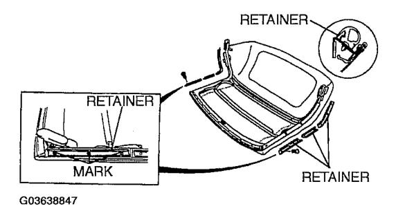
Fig. 44: Installing Retainers To Link Courtesy of MAZDA MOTORS CORP.
