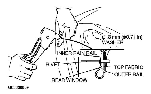
Fig. 56: Riveting Rain Rail To Top Fabric Courtesy of MAZDA MOTORS CORP.
