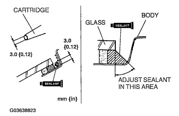
Fig. 20: Reshaping Sealant Courtesy of MAZDA MOTORS CORP.
