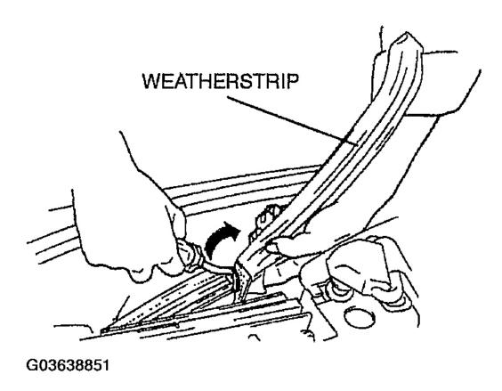
Fig. 48: Removing Fastener Courtesy of MAZDA MOTORS CORP.
