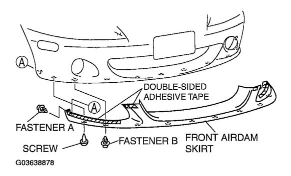
Fig. 75: Removing Front Airdam Skirt (BP With TC) Courtesy of MAZDA MOTORS CORP.
