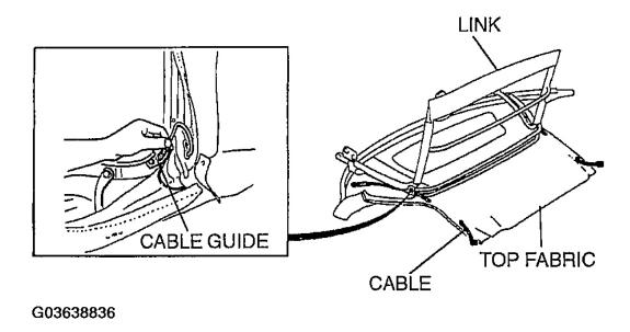
Fig. 33: Removing Top Fabric And Cables From Link Courtesy of MAZDA MOTORS CORP.
