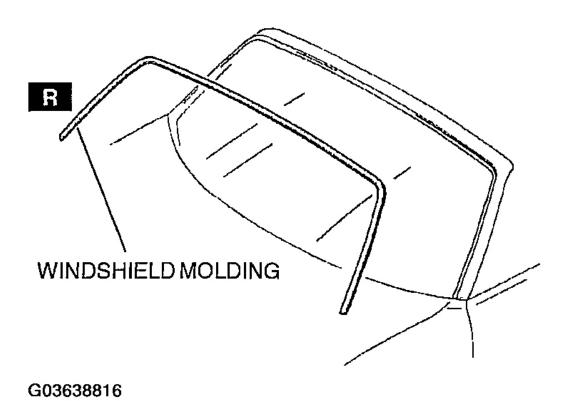
Fig. 13: Removing Windshield Molding From Windshield Courtesy of MAZDA MOTORS CORP.
