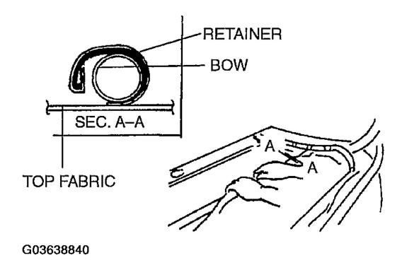
Fig. 37: Assembling Top Fabric To Bow Retainer Courtesy of MAZDA MOTORS CORP.
