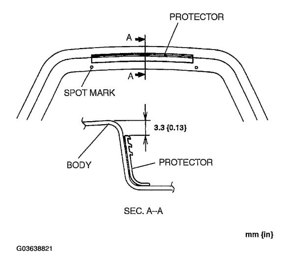
Fig. 18: Bonding Protector To Body Courtesy of MAZDA MOTORS CORP.
