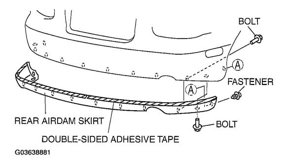
Fig. 78: Removing Rear Airdam Skirt (BP With TC) Courtesy of MAZDA MOTORS CORP.
