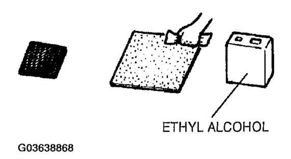
Fig. 65: Degreasing Repair Sheets Using Ethyl Alcohol Courtesy of MAZDA MOTORS CORP.
