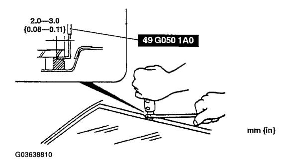
Fig. 7: Cutting Sealant Near Glass (1 Of 2) Courtesy of MAZDA MOTORS CORP.
