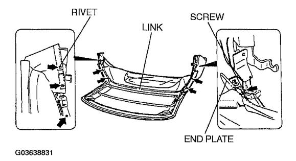
Fig. 28: Disassembling End Plate Courtesy of MAZDA MOTORS CORP.
