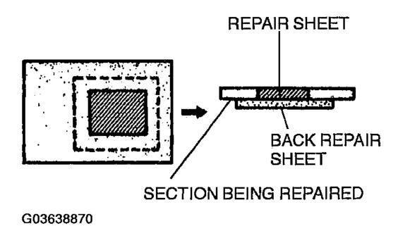
Fig. 67: Pressing Repair Sheets Together Courtesy of MAZDA MOTORS CORP.
