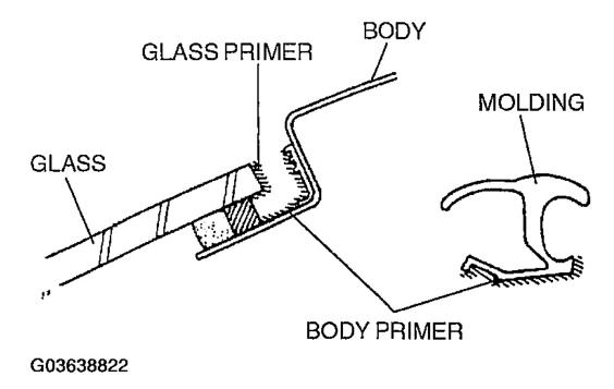
Fig. 19: Apply Primer Onto Bonding Area Of Glass Courtesy of MAZDA MOTORS CORP.
