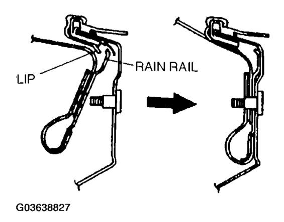
Fig. 24: Inserting Rain Rail Into Beltline Molding Lip Courtesy of MAZDA MOTORS CORP.
