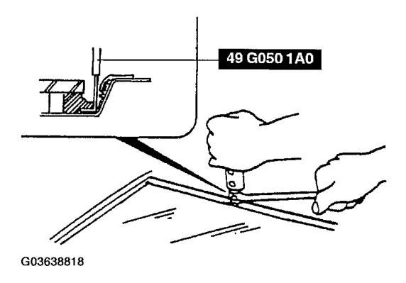
Fig. 15: Cutting Sealant Near Body Courtesy of MAZDA MOTORS CORP.
