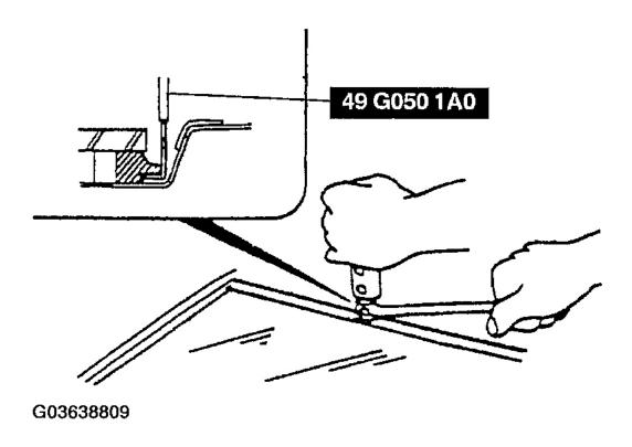
Fig. 6: Cutting Sealant Near Body Courtesy of MAZDA MOTORS CORP.
