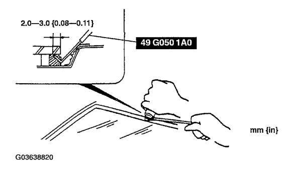
Fig. 17: Cleaning Around Edge Of Glass Courtesy of MAZDA MOTORS CORP.
