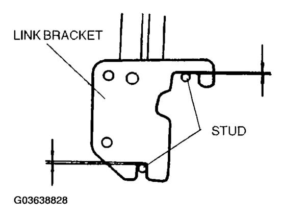
Fig. 25: Installing Link Bracket Over Studs Courtesy of MAZDA MOTORS CORP.
