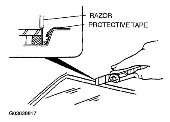
Fig. 14: Cutting Sealant Using Razor Courtesy of MAZDA MOTORS CORP.
