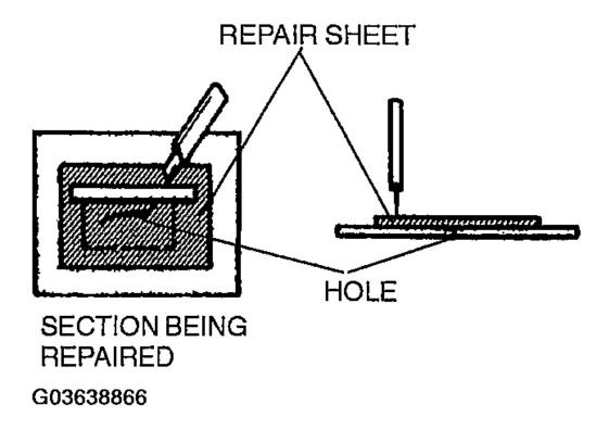
Fig. 63: Placing Repair Sheet Over Damaged Section Courtesy of MAZDA MOTORS CORP.
