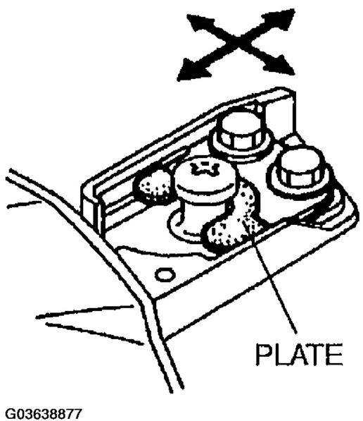
Fig. 74: Tightening Plate Courtesy of MAZDA MOTORS CORP.
