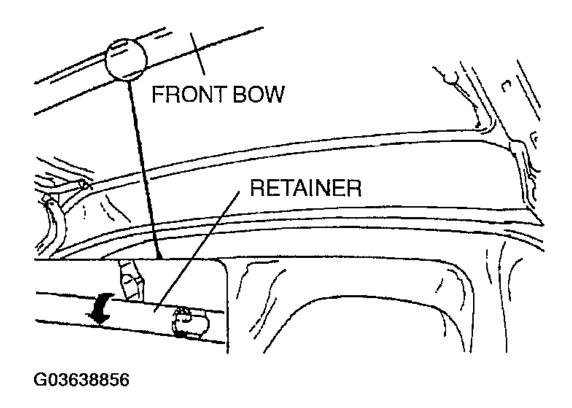
Fig. 53: Removing Top Fabric From Bow Retainer Courtesy of MAZDA MOTORS CORP.
