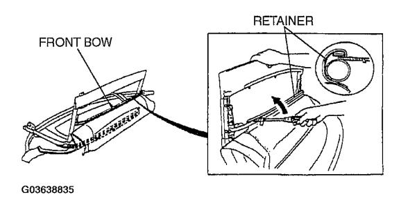
Fig. 32: Removing Top Fabric From Bow Retainer Courtesy of MAZDA MOTORS CORP.
