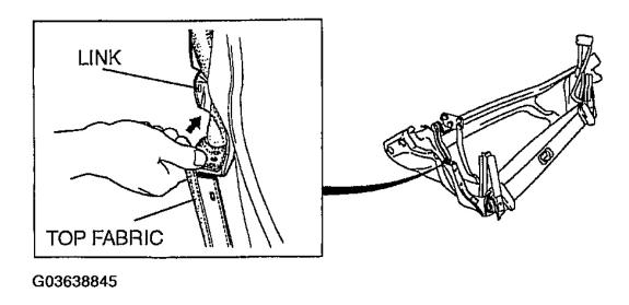
Fig. 42: Installing Top Fabric To Link Courtesy of MAZDA MOTORS CORP.
