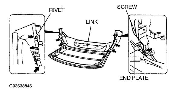
Fig. 43: Riveting Top Fabric To Link Courtesy of MAZDA MOTORS CORP.
