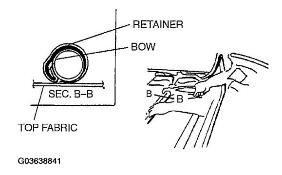
Fig. 38: Clamping Top Fabric To Bow Courtesy of MAZDA MOTORS CORP.
