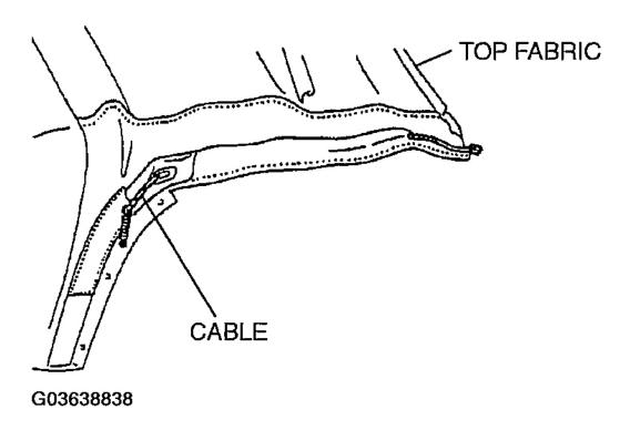
Fig. 35: Threading Cable Into Top Fabric Courtesy of MAZDA MOTORS CORP.
