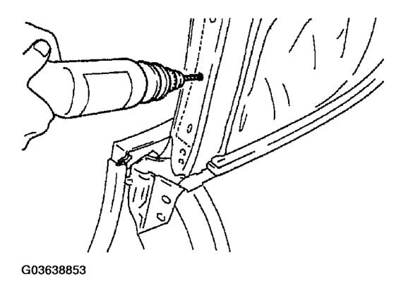
Fig. 50: Removing Rivets From Link Using Drill Courtesy of MAZDA MOTORS CORP.
