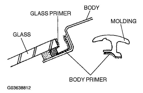
Fig. 9: Applying Primer Onto Bonding Area Of New Rear Window Molding Courtesy of MAZDA MOTORS CORP.
