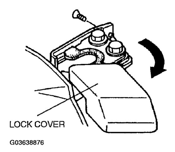
Fig. 73: Opening Lock Cover Courtesy of MAZDA MOTORS CORP.
