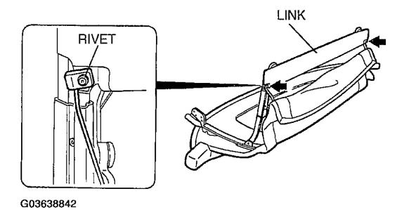
Fig. 39: Riveting Cables To Front Of Link Courtesy of MAZDA MOTORS CORP.
