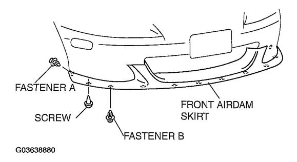
Fig. 77: Installing Front Airdam Skirt (BP With TC) Courtesy of MAZDA MOTORS CORP.
