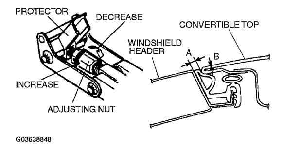
Fig. 45: Adjusting Convertible Top Courtesy of MAZDA MOTORS CORP.
