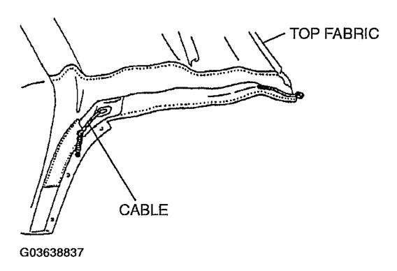
Fig. 34: Removing Cables From Top Fabric Courtesy of MAZDA MOTORS CORP.
