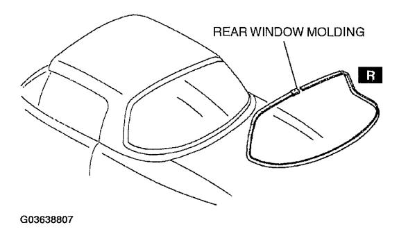
Fig. 4: Removing Rear Window Molding Courtesy of MAZDA MOTORS CORP.
