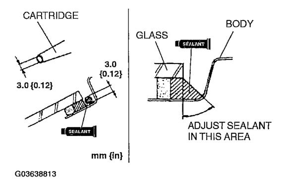
Fig. 10: Reshaping Sealant Courtesy of MAZDA MOTORS CORP.
