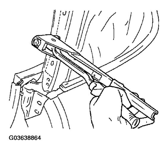
Fig. 61: Riveting Top Fabric Upper Side To Link Courtesy of MAZDA MOTORS CORP.
