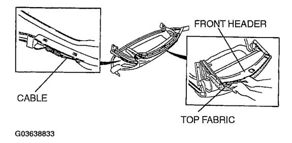
Fig. 30: Disconnecting Cables From Rear Of Link Courtesy of MAZDA MOTORS CORP.
