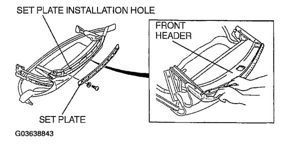
Fig. 40: Installing Set Plate To Link Courtesy of MAZDA MOTORS CORP.
