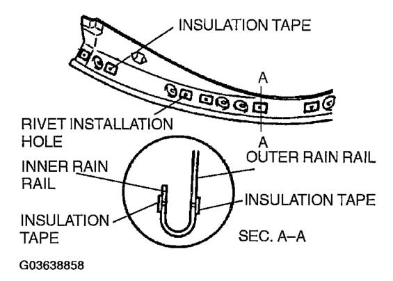
Fig. 55: Installing Insulation Tape To Rivet Installation Holes Of Rain Rail Courtesy of MAZDA MOTORS CORP.
