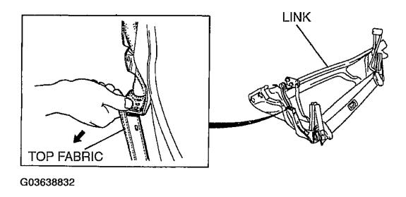
Fig. 29: Removing Top Fabric From Link Courtesy of MAZDA MOTORS CORP.
