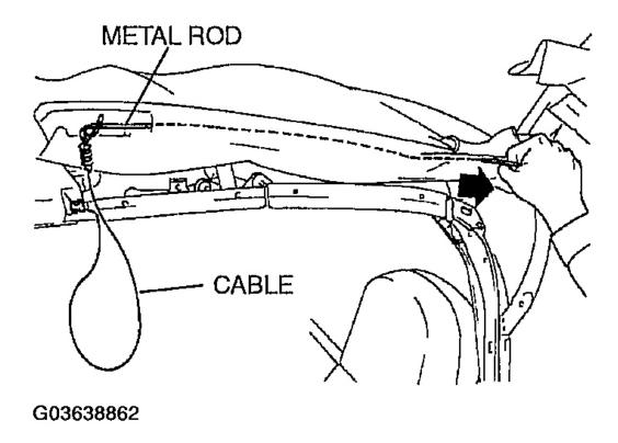
Fig. 59: Inserting A Metal Rod Into Fabric Courtesy of MAZDA MOTORS CORP.
