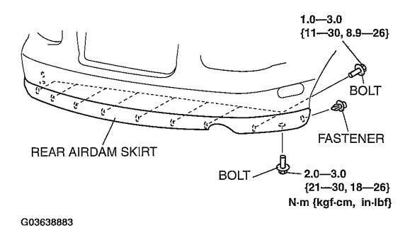
Fig. 80: Installing Rear Airdam Skirt (BP With TC) - With Torque Specifications Courtesy of MAZDA MOTORS CORP.
