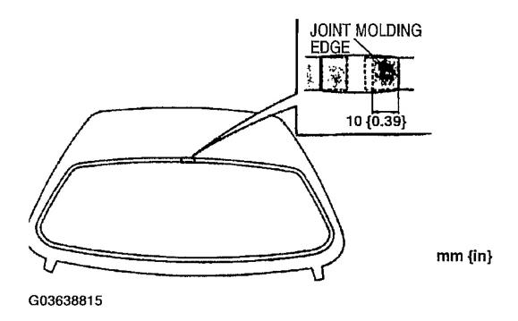
Fig. 12: Identifying Joint Molding Edge Specification Courtesy of MAZDA MOTORS CORP.
