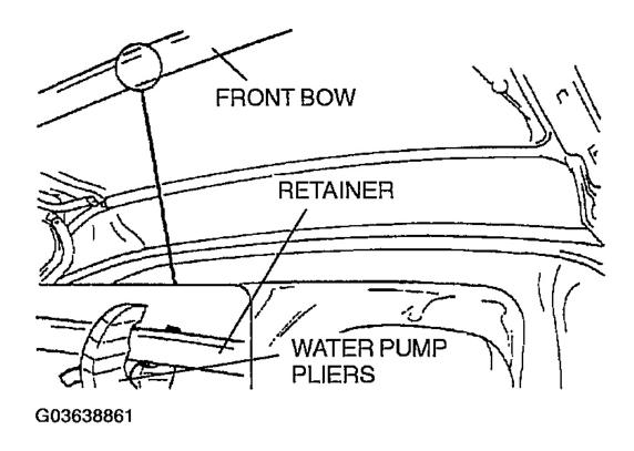
Fig. 58: Clamping Top Fabric To Bow Courtesy of MAZDA MOTORS CORP.
