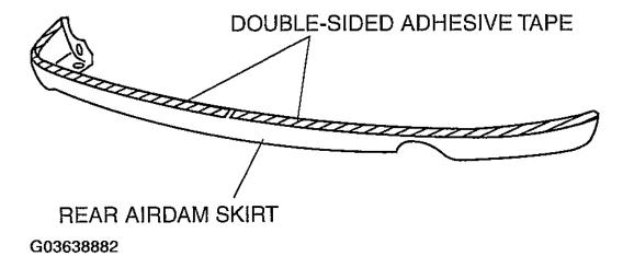
Fig. 79: Affixing Double-Sided Adhesive Tape To Rear Airdam Skirt Courtesy of MAZDA MOTORS CORP.
