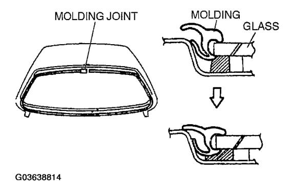
Fig. 11: Installing Rear Window Molding With Molding Joint At Top Courtesy of MAZDA MOTORS CORP.
