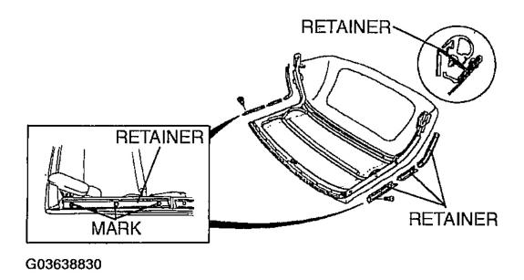
Fig. 27: Disassembling Retainer Courtesy of MAZDA MOTORS CORP.
