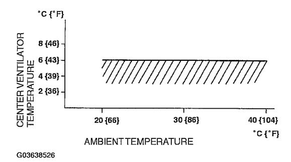
**<u>Fig. 3: Refrigerant System Performance Test Graph</u> Courtesy of MAZDA MOTORS CORP.**
